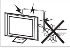
High voltages are used in the operation of this television receiver. Do not remove the cabinet back from your set. Refer servicing to qualified service personnel.
