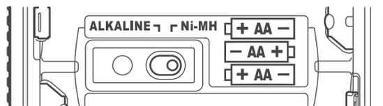
1. Remove the battery cover and set the battery switch.
