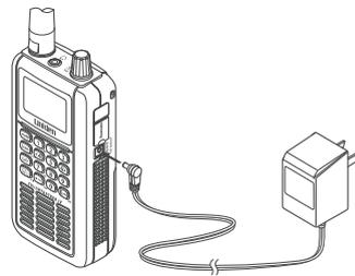
If rechargeable batteries are installed and **ALKALINE/Ni-MH** is set to **Ni-MH**, the adaptor powers the scanner and recharges the installed batteries at the same time.
