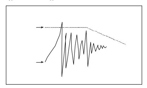
On the other hand, this chart shows the same hit but with the Decay parameter set at a higher value. Notice how the Decay threshold is slightly higher and stays consistent for a longer time before it tapers off. Now only the initial strike of the drum triggers the DM5.
