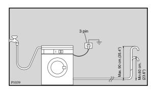
When discharging into a standpipe ensure that the top of the curve in the hose end is no more than 90cm (35.4") and no less than 60cm (23.6") above floor level. The upright standpipe should have a minimum length of 30cm (12") from the bottom of the elbow to the top of the pipe (see diagram).
