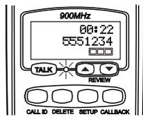
To answer a call if the handset is on the base, lift the handset and press **TALK**. Or, if the handset is away from the base, press any key on the handset before speaking. The TALK indicator on the handset lights and the IN USE indicator on the base flashes.
