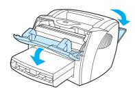
2 Rotate the green pressure release levers downward. If you can remove the media without removing the print cartridge, do so, and continue with step 4.
