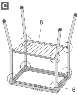
Repeat step B on the opposite corner of the storage rack (8) so that it is horizontally stable. Finally, fix the other two corners of the storage rack (8).
