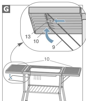
To place the folding trays (10) in the horizontal position, lift the tray and latch the wire support strut (9) into the catch provided for this purpose.
