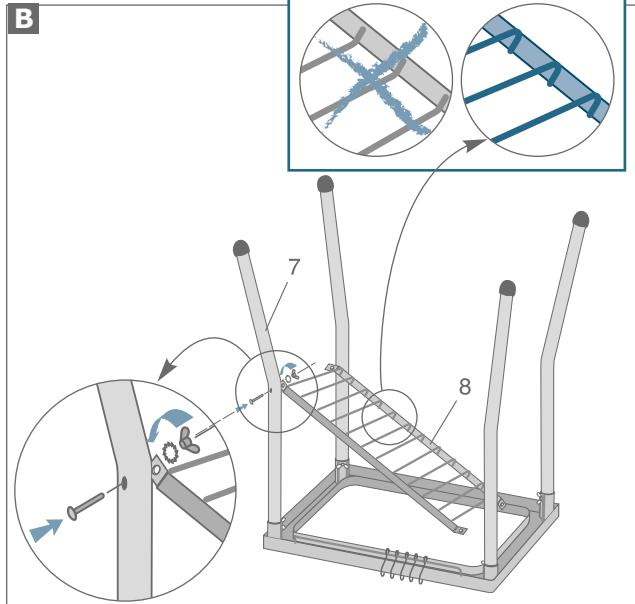
Insert a bolt into the leg (7), from the outside, then add a washer and tighten using a butterfly nut, trapping a corner of the storage rack (8).
