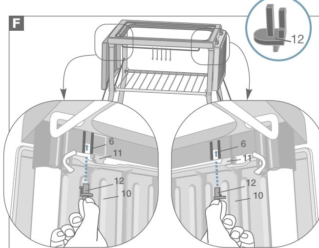
For each folding tray (10), lock the front hinge by inserting a locking clip (12). Fit it between the two guide grooves provided for this purpose on the edge of the support frame (6).
