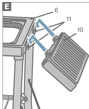
Insert the folding trays (10) on either side of the support frame (6), in the notches provided for this purpose (11).
