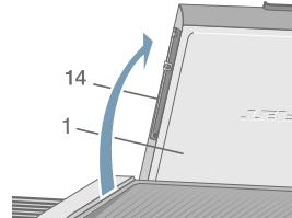
Remove the protective cover (1) from the appliance by opening it to mid-height and then lifting it from the back of the appliance.
