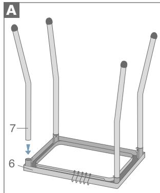
Place the support frame (6) upside down on a flat, stable surface. Insert the four legs (7) in the support frame (6) without tightening the butterfly nuts.
