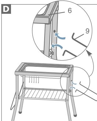
Turn over the assembly. Insert the wire support struts (9) into the legs, on either side of the support frame (6).
