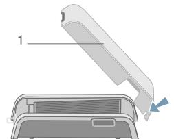
Insert the protective cover (1) at the back of the appliance, as shown in the drawing opposite.
