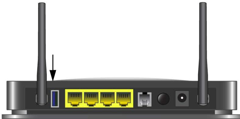
**Figure 8. USB port on rear panel.**
