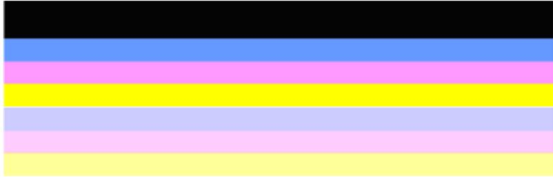
Example of Good Color Bars: All bars are solid, sharp-edged, and extend with uniform color across the entire page. The printer is operating correctly.
