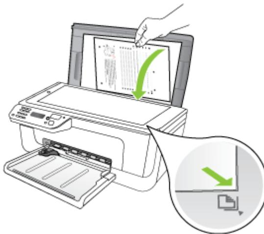
5. Press **OK** to scan the alignment sheet.
