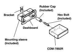
Remove the Detachable Front Panel (refer to page 4). Slide mounting sleeve from main unit (see Removal Procedure below). Slide the mounting sleeve into the dashboard.
