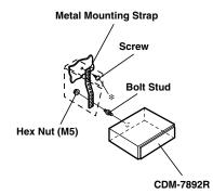
When your vehicle has the Bracket, mount the long hex bolt onto the rear panel of the CDM-7892R and put the Rubber Cap on the hex bolt. If your vehicle does not have the Mounting Support, reinforce the head unit with the metal mounting strap (not supplied). Connect all the leads of the CDM-7892R according to details described in the CONNECTIONS section.
