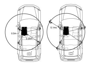
Here we calculate the time correction value for the front left speaker in the diagram at the left.
