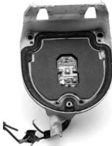
6. Squeeze the primer tube to break the glass bulb and wet the brush end with primer. Rub the primer on the housings at the places where the tape will touch. Treat all tail light housings at the same time before the primer tube dries out.
