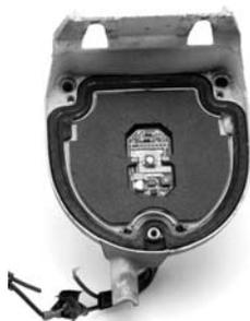
10. Reinstall the tail light lenses and secure with the lens screws.
