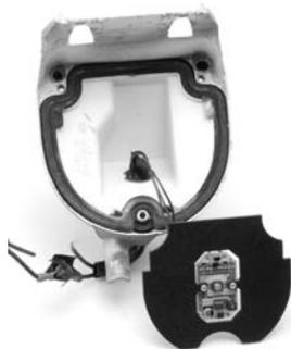
9. Remove the backing from the tape on the LED assembly and insert assembly into the tail light housing, making sure to keep the assembly centered in housing. Press firmly on the bracket to ensure good tape bonding.
