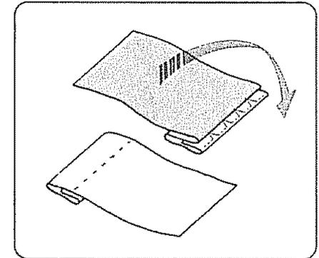
There are two blind hem stitches on your machine. The regular blind hem is used for woven fabrics. The stretch blind hem is wider and will "give" and is used for knit and stretch fabrics.
