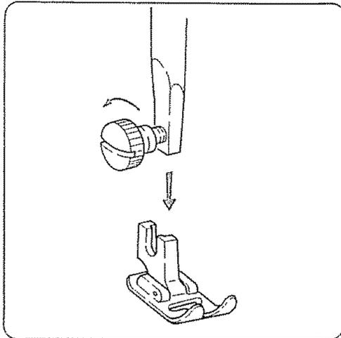
To change the various presser feet, raise the presser bar to its highest position by lifting the presser foot lever. Loosen the presser foot thumb screw, choose the proper foot, insert from the bottom. Tighten the screw using the large screw driver to make certain the foot is secure.
