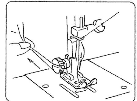
3. Pull both threads under and to the back of the presser foot, leaving 3 to 4 inches of thread clear.
