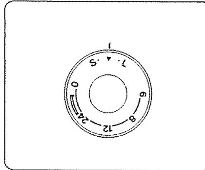
In stretch stitch sewing, Stitch Length Control should be in the detent position between S and L (▼ position) for most materials. Depending upon the type of fabric used, you may need to adjust this control to match forward stitches of stretch sewing with reverse motion stitches. To shorten stretch stitches, turn the control slightly toward "S". To lengthen, turn toward "L".
