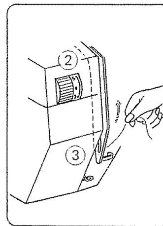
2. While holding thread near spool, draw thread into threading channel toward you making sure the thread is pulled firmly between the tension discs.
