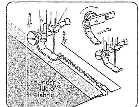
4. To sew the left side of the zipper, set the zipper foot on the left side of the needle.
