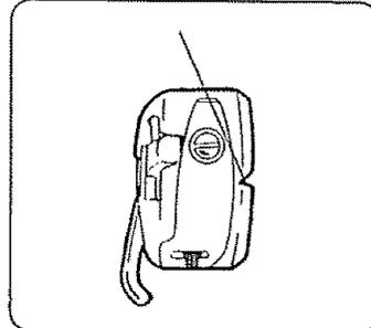
Pull thread through slot of case as shown.
