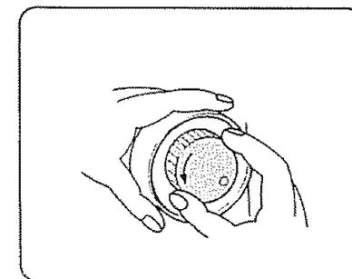
Release clutch by turning the clutch knob inside the hand wheel toward you.
