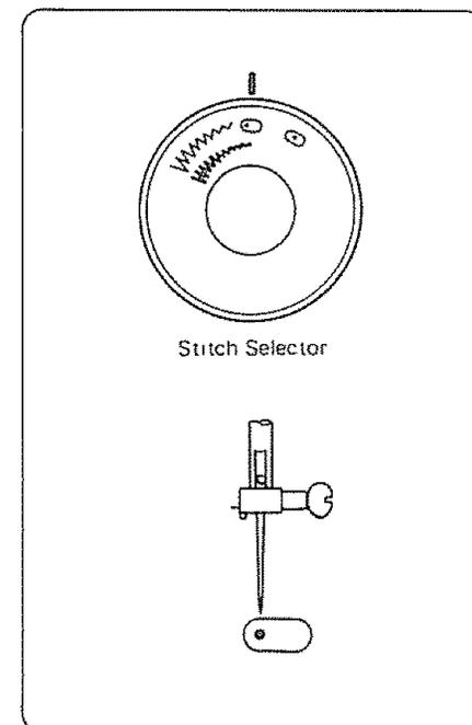
Use Left Needle Position for more control while topstitching or edge stitching difficult fabrics.
