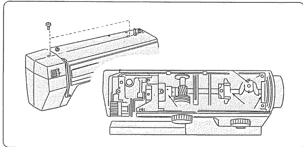
Remove top cover plate to oil points indicated in top of machine head. To remove cover plate, loosen up two top screws and lift the cover plate as illustrated.
