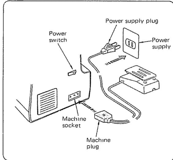
**NOTE:** Before inserting the plug into your machine, be sure the power switch is OFF.
