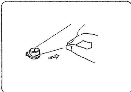
Draw thread from spool through bobbin winder tension disc as shown.
