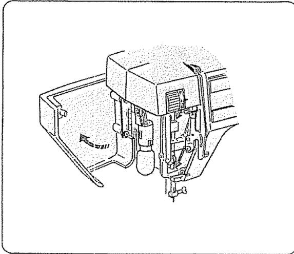
Open face cover plate and oil points in illustration. Use only a drop of oil; do not over-oil.
