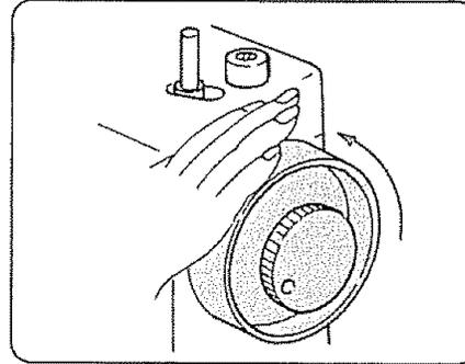
1. Raise presser foot lever. Hold needle thread loosely in left hand and rotate handwheel toward you one complete turn.
