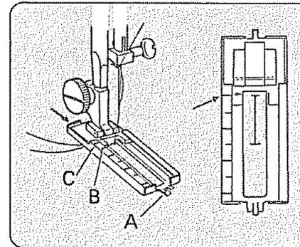
2. a. Move the slider (A) toward you so that the top mark (C) on the slider meets the start mark (B).
