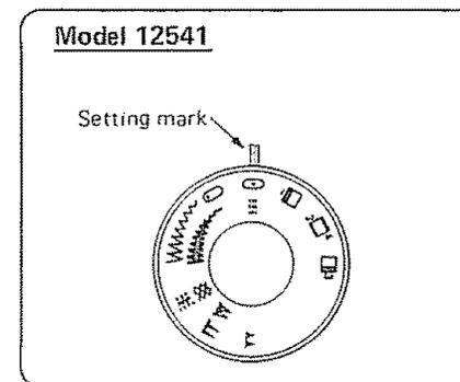
The stitch selector control not only determines the stitch you select, but also regulates the stitch width for regular zigzag and rick rack stretch stitches.
