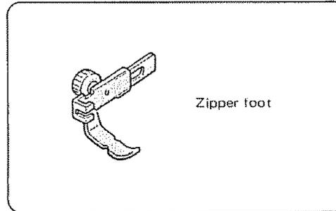
This foot can be set to sew on each side of your zipper. The edges of the foot guide the zipper and keep the seam straight.
