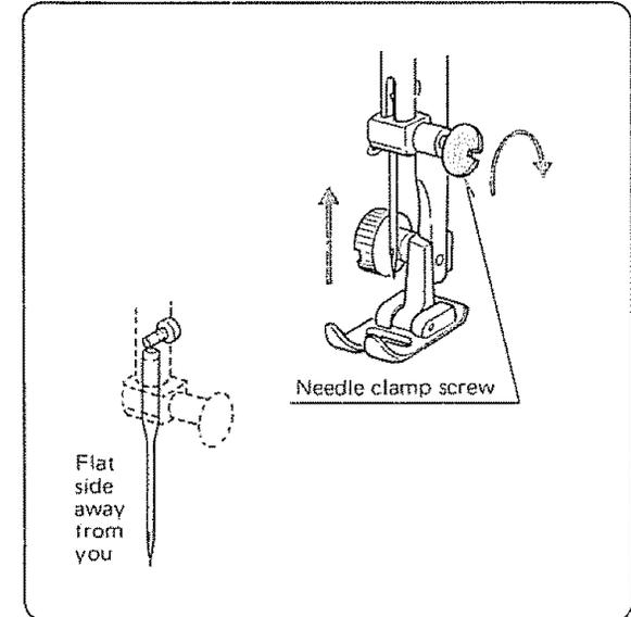
**NOTE:** Raise the needle bar to its highest position by turning the hand wheel toward you.
