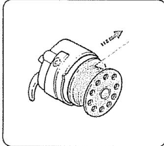
Place bobbin in bobbin case making sure thread feeds clockwise and is coming from bobbin as shown.
