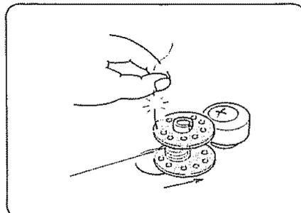
Place bobbin onto bobbin winder spindle with end of thread coming from the top of the bobbin. Push bobbin winder shaft to the right until it clicks. Holding onto end of thread, start machine. When bobbin is slightly filled, snip off end of thread.
