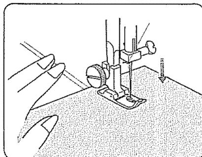
Before sewing with the straight stitch foot, be sure the stitch selector dial is set to the center needle position.
