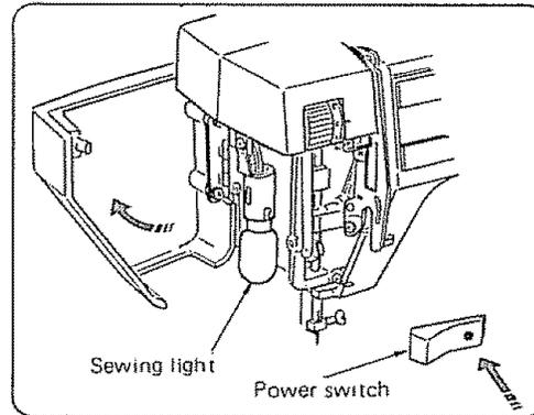
4. Push the light and power switch to turn on the power and sewing light.
