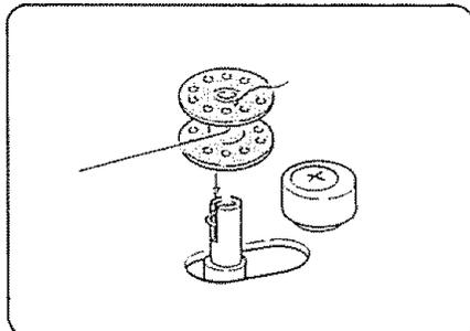
Pull end of thread through hole in bobbin as shown.
