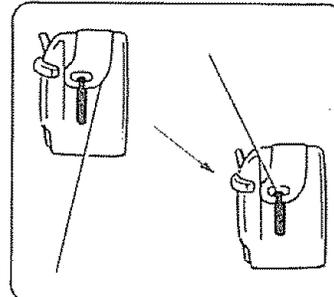
Pull thread under tension spring and through the opening as shown above.
