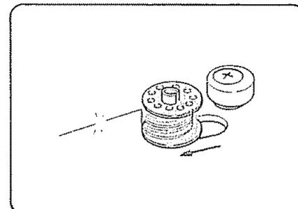
Wind thread until winder stops. Remove bobbin. Clip thread.
