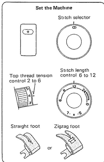
**NOTE:** Best sewing results are obtained with the straight stitch foot, but the zigzag foot will also provide acceptable results.
