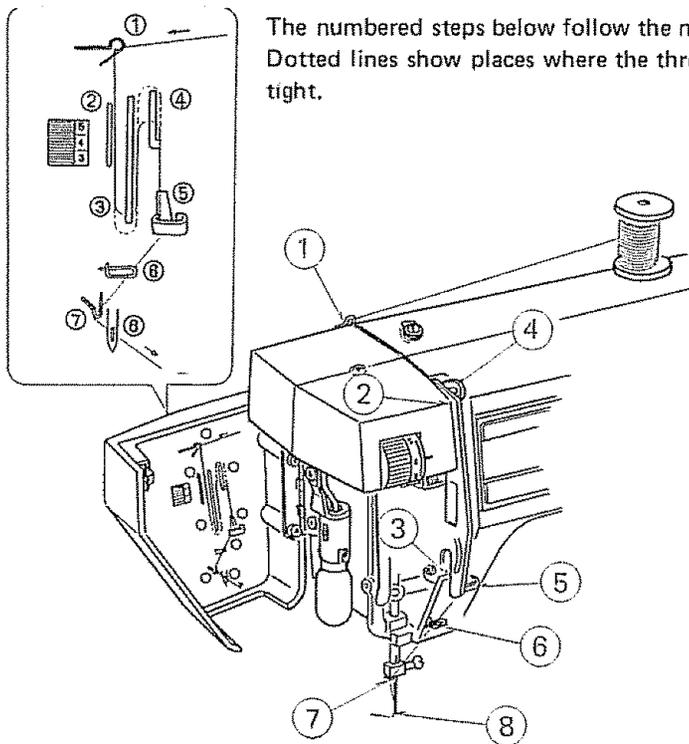
The numbered steps below follow the numbers on the illustrations. Dotted lines show places where the thread loops and then is pulled tight.
