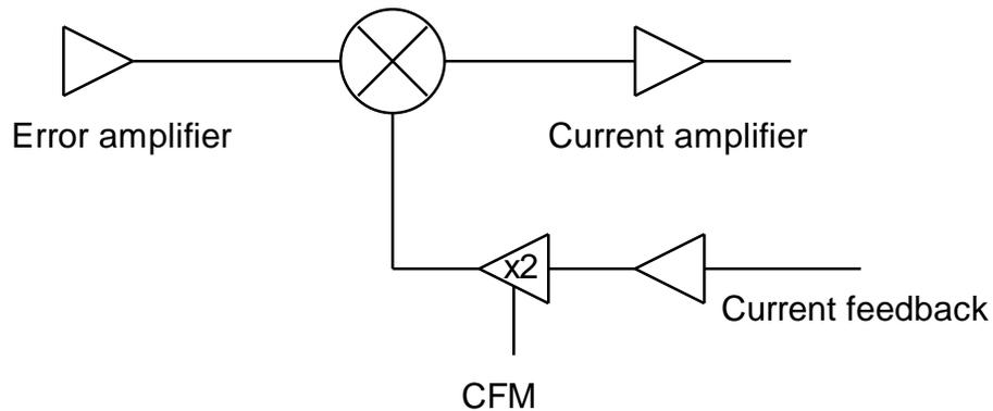
The amplifier is equipped with a Current Feedback Multiplier (CFM). By turning DIP switch 2 (on the upper board of the power stage) to ON, the signal of the current feedback is multiplied by 2 and consequently the following changes occur:
