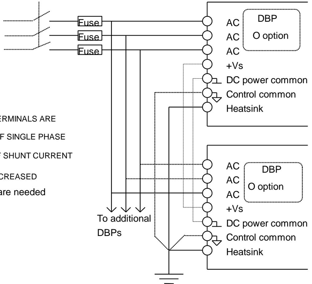
NOTE: DC POWER TERMINALS ARE CONNECTED IF SINGLE PHASE IS USED OR IF SHUNT CURRENT HAS TO BE INCREASED
