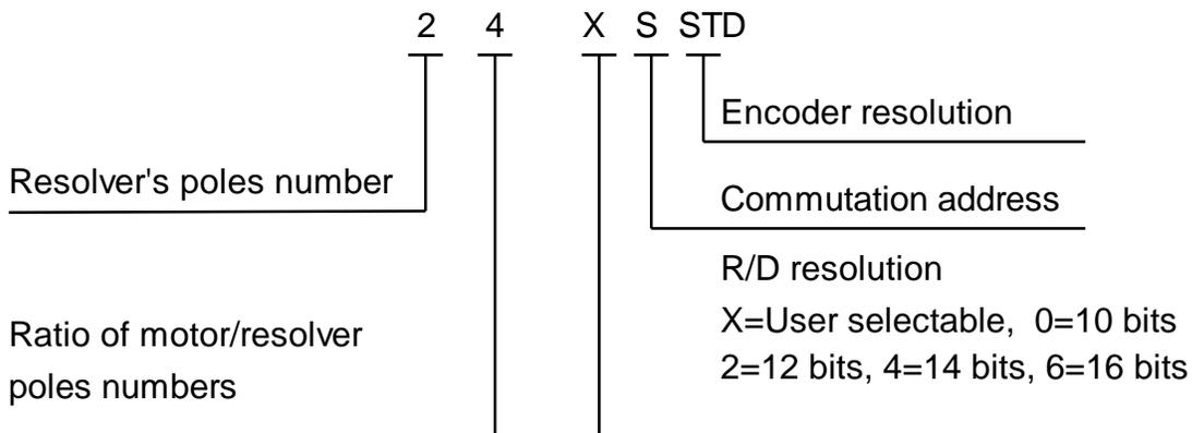
In the S (standard) version zero crossing of phases B C occurs at position address "0" of the Resolver.
