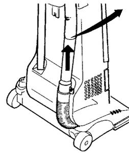
1. Remove the attachment hose from the lower hose retainer and look into the hose retainer for any obstructions. Proceed to Step 2 to check for any other blockages.
