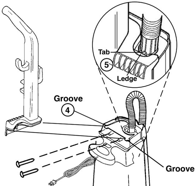
4. From rear of cleaner, align handle with groove and slide onto cleaner. If necessary, use thumb and finger pressure to slide handle into position.
