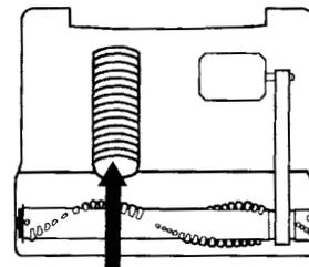
4. Check for blockages in the brush roll area and remove any obstructions found there. The base hose can be cleared of any blockage by using a blunt instrument.
