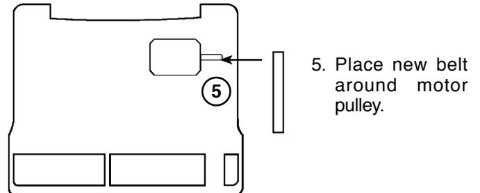
5. Place new belt around motor pulley.
