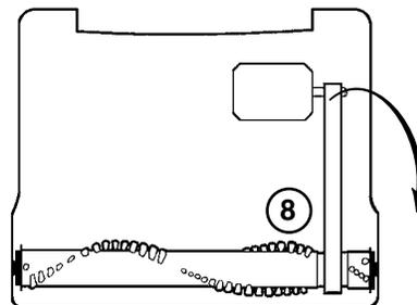
8. Pull right side of brush roll to stretch belt. Secure right end cap into base.
