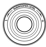
When using the remote control, press **SUBWOOFER LEVEL +** to increase the subwoofer volume or press **SUBWOOFER LEVEL -** to decrease it.
