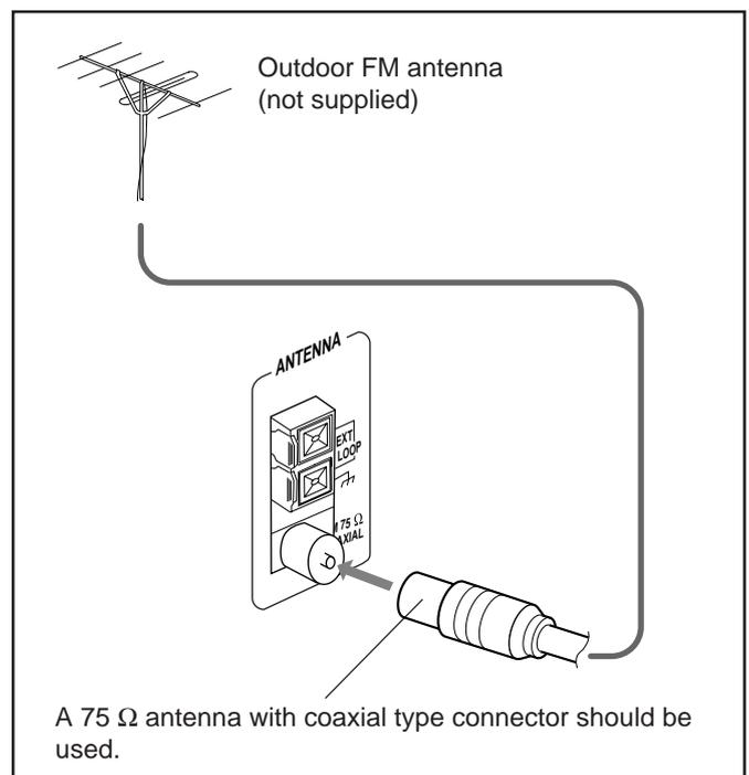
A 75 Ω antenna with coaxial type connector should be used.
