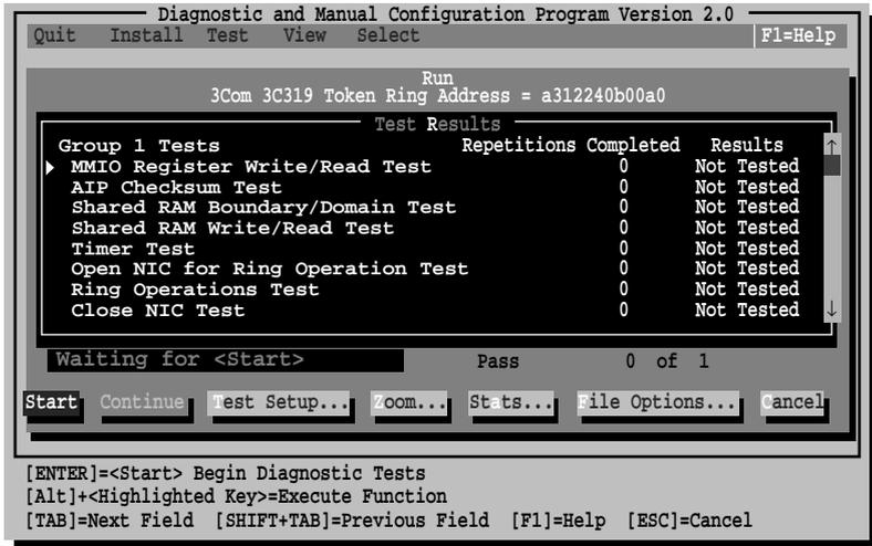
Figure 9-3 Run Tests Dialog Box
