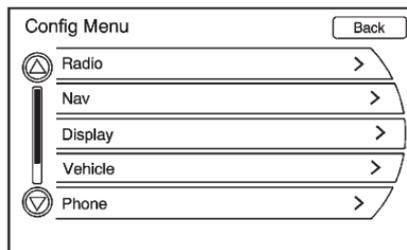
To access the Radio settings menu, press CONFIG to display the Config Menu. Turn the MENU/SELECT knob to scroll through the available features until the Radio feature displays. Press this feature to display more options.
