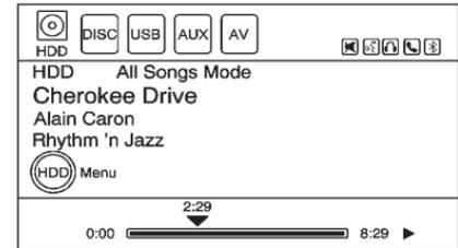
Press CD/AUX/HDD, cycle through the available audio source until the HDD source displays or press CD/AUX/HDD once, and then press the HDD source button.
