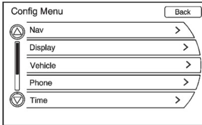
1. Press the CONFIG control button. Turn the MENU/SELECT knob until the Phone menu displays. Press the MENU/SELECT knob to display other phone options.
