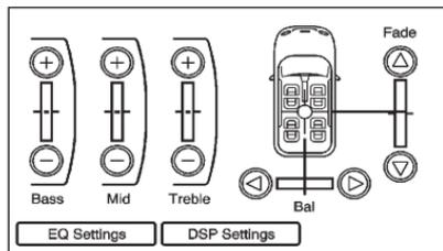
To view the DSP options, press the DSP Settings screen button on the Sound Menu.
