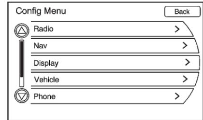
Press CONFIG to enter the Config setup menu features. Turn the MENU/SELECT knob until the Display feature displays. Press the MENU/SELECT knob or press the Display screen button to display the other options.
