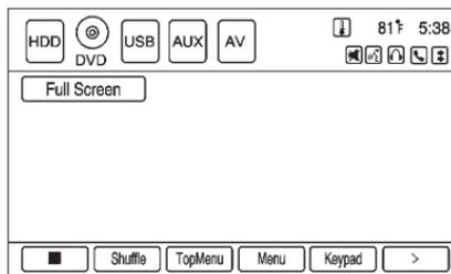
To view the DVD video, the vehicle must be in P (Park) for an automatic transmission or the parking brake must be engaged for a manual transmission.
