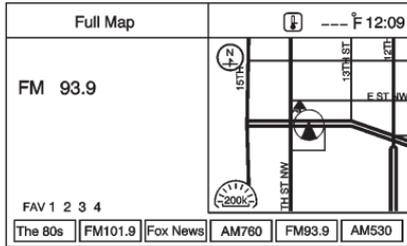
Press the audio display screen button to display the current audio source screen. The display shows a split screen with the audio source screen on the left side and the map or guidance screen on the right side. Press the Full Map screen button to exit the split view screen.
