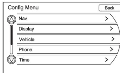
Turn the MENU/SELECT knob to scroll through the available setup features. Once the desired feature displays, press the MENU/SELECT knob or press the desired feature on the screen, to display more options within that feature.
