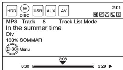
If a disc is already loaded, but you are currently on a map screen or listening to a different audio source, press CD/AUX/HDD to switch to the Disc source. A track number appears on the display when each track starts to play.
