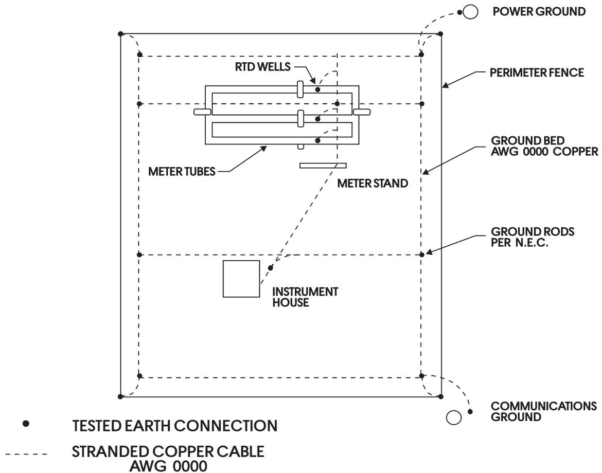
Figure 2 Overhead Map of Ground Bed for Gas Metering Station
