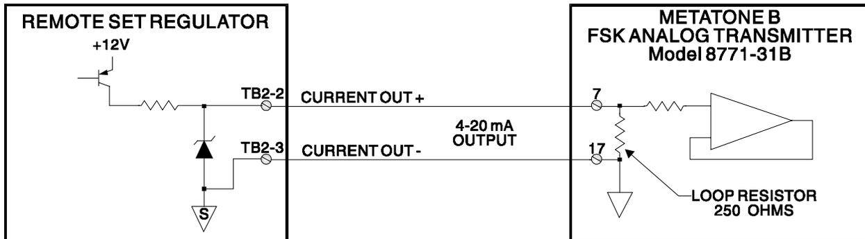
Figure 4-6 - Current Output to FSK Bi-State Transmitter
