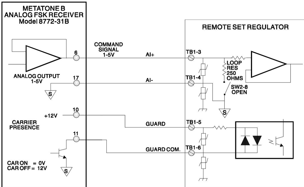
Figure 4-2 - Analog Voltage Input with Guard
