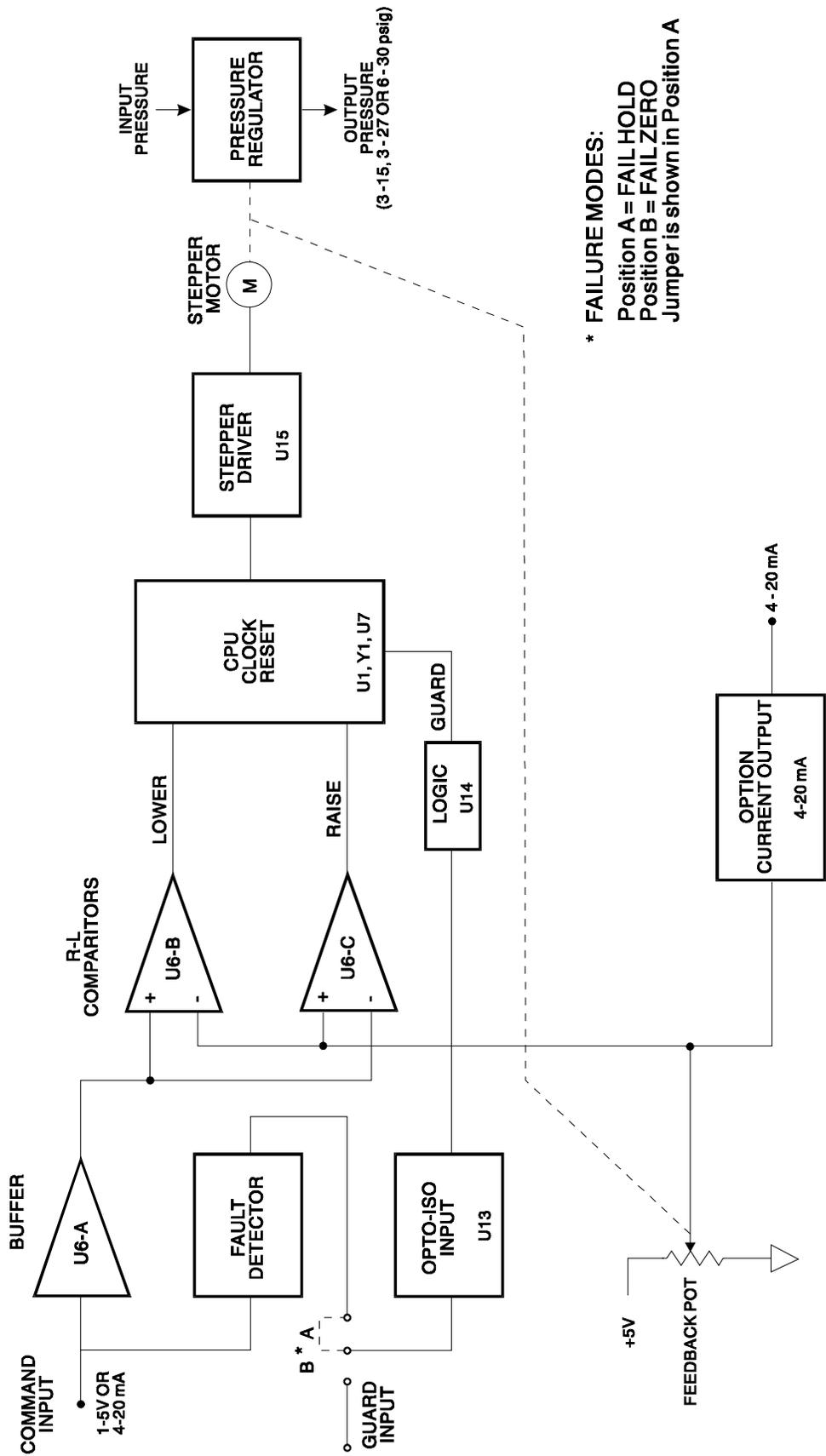
Figure 1-2 - Block Diagram of Analog Type Regulator
