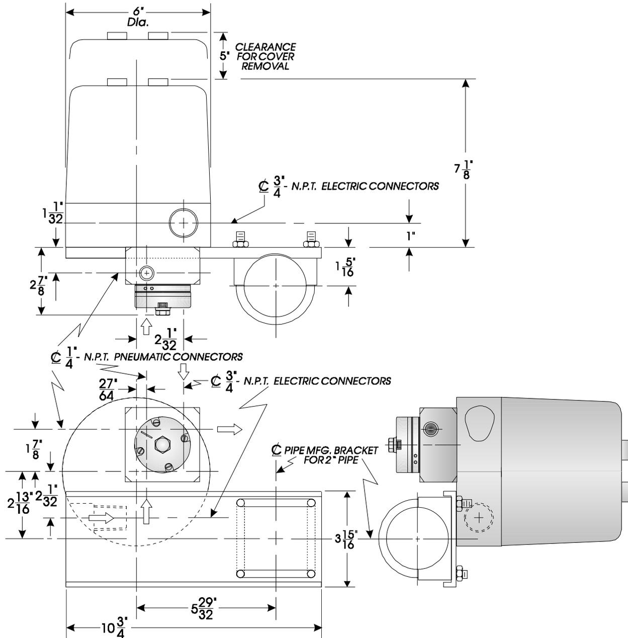
Figure 2-1 - Overall Mounting Dimensions
