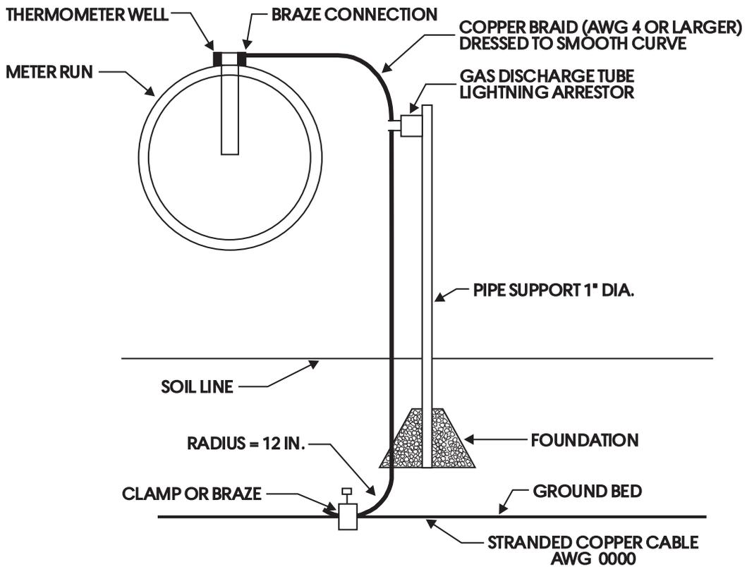
Figure 6 Grounding of Thermometer Well in Gas Line
