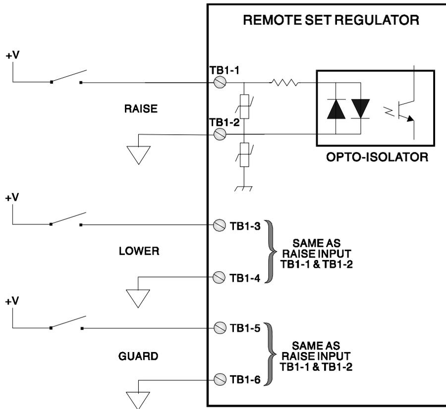
Figure 4-5 - Raise/Lower & Guard Inputs from Relay Contacts
