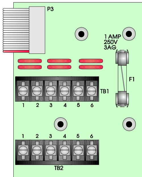
Figure 5-7 - Assembly, Raise/Lower Termination Board
