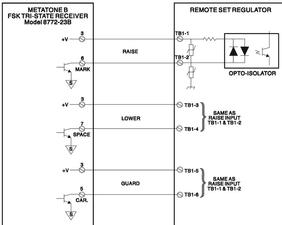
Figure 4-5 - Raise/Lower & Guard Inputs from Open Collectors
