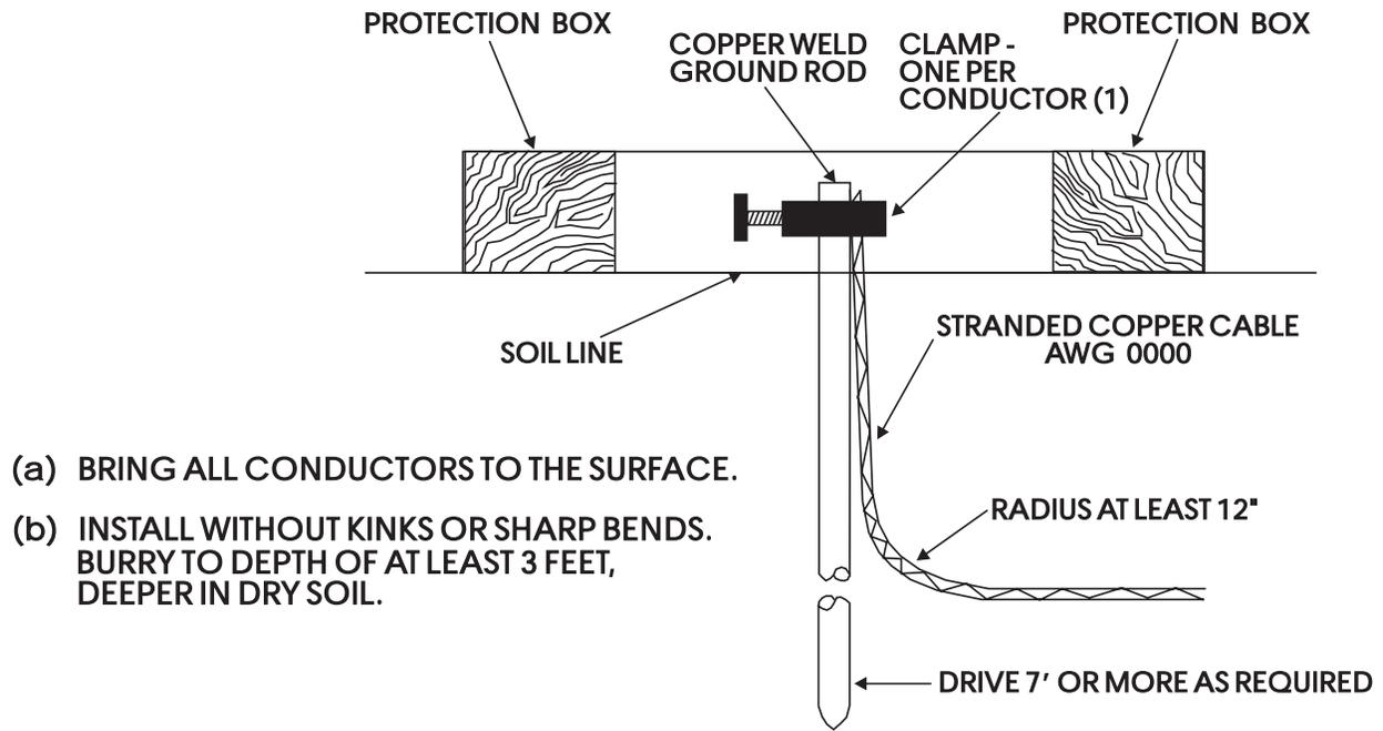
Figure 1 Basic Ground Rod Installation
