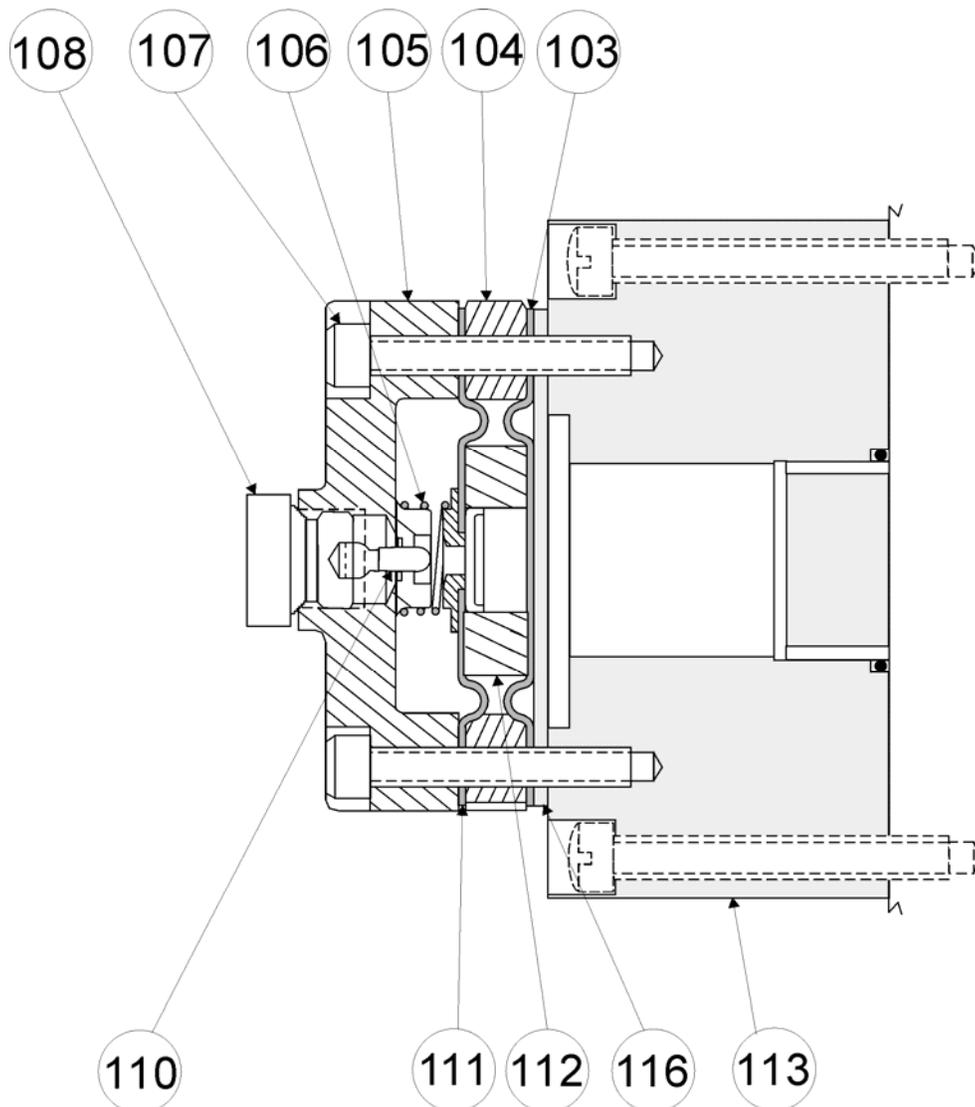
Figure 7-3 – Remote Set Regulator Assembly Basic Parts
