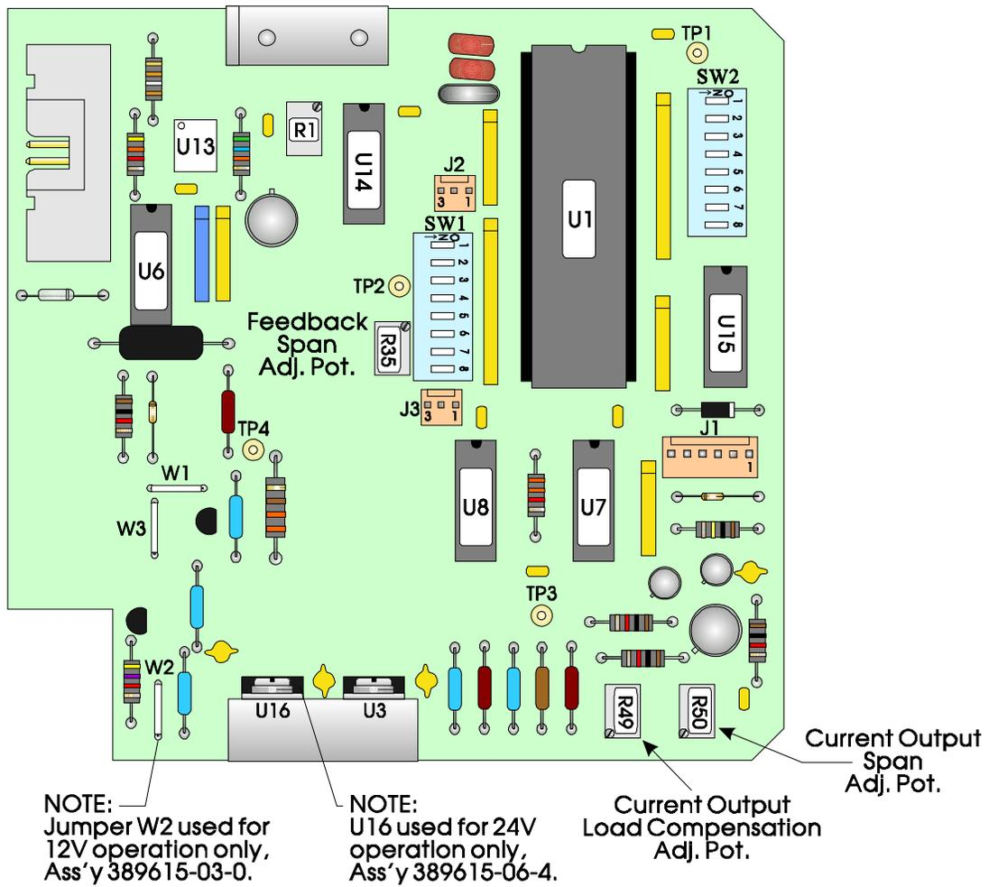
Figure 5-4 - Assembly, Analog Type CPU Board with Current Output
