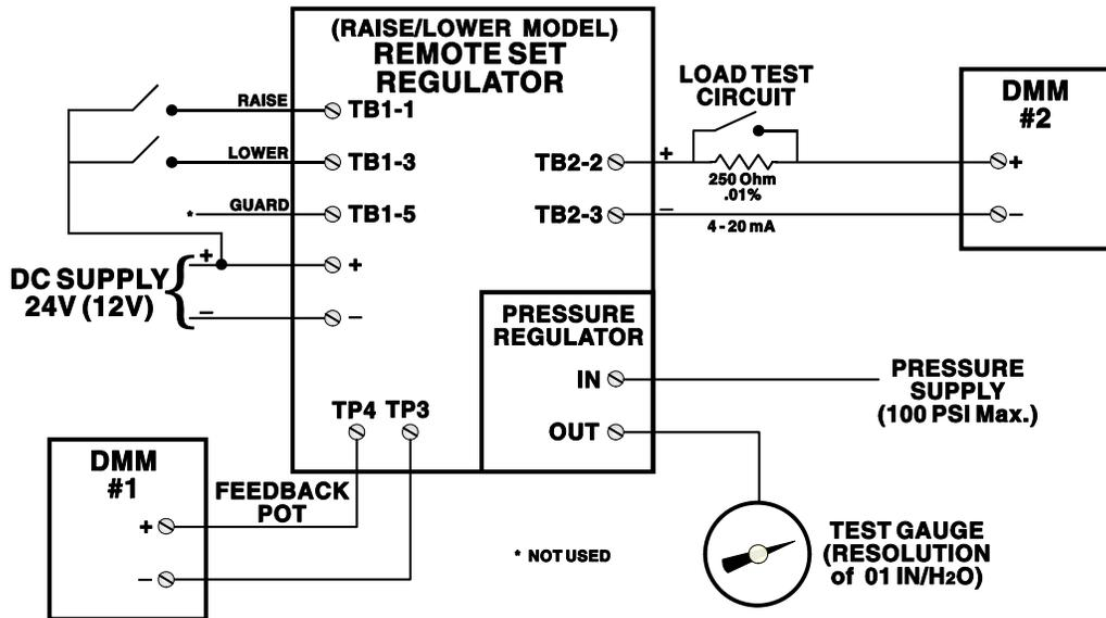
Figure 5-3 - Raise/Lower Test Setup
