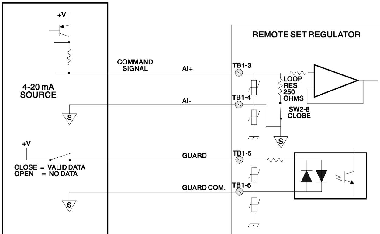
Figure 4-3 - Analog Current Input with Guard
