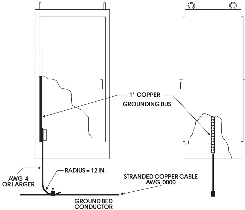
**Figure 3 Grounding of Equipment Housing**
