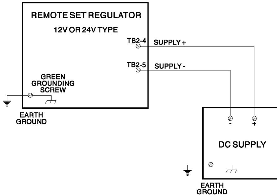
Figure 4-7 - DC Supply Connections
