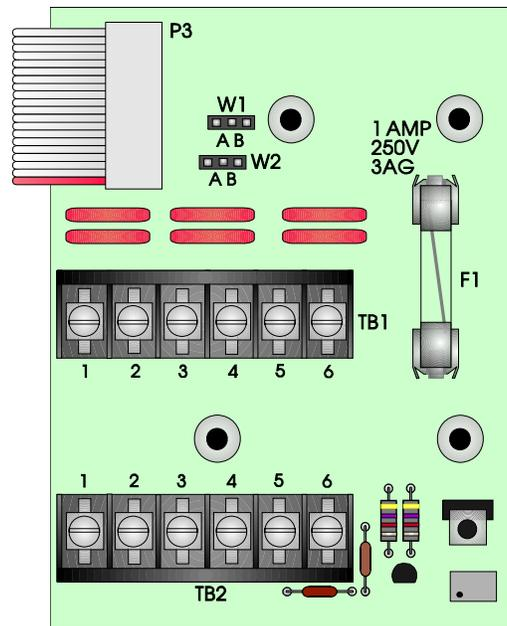
Figure 5-5 - Assembly, Analog Termination Board
