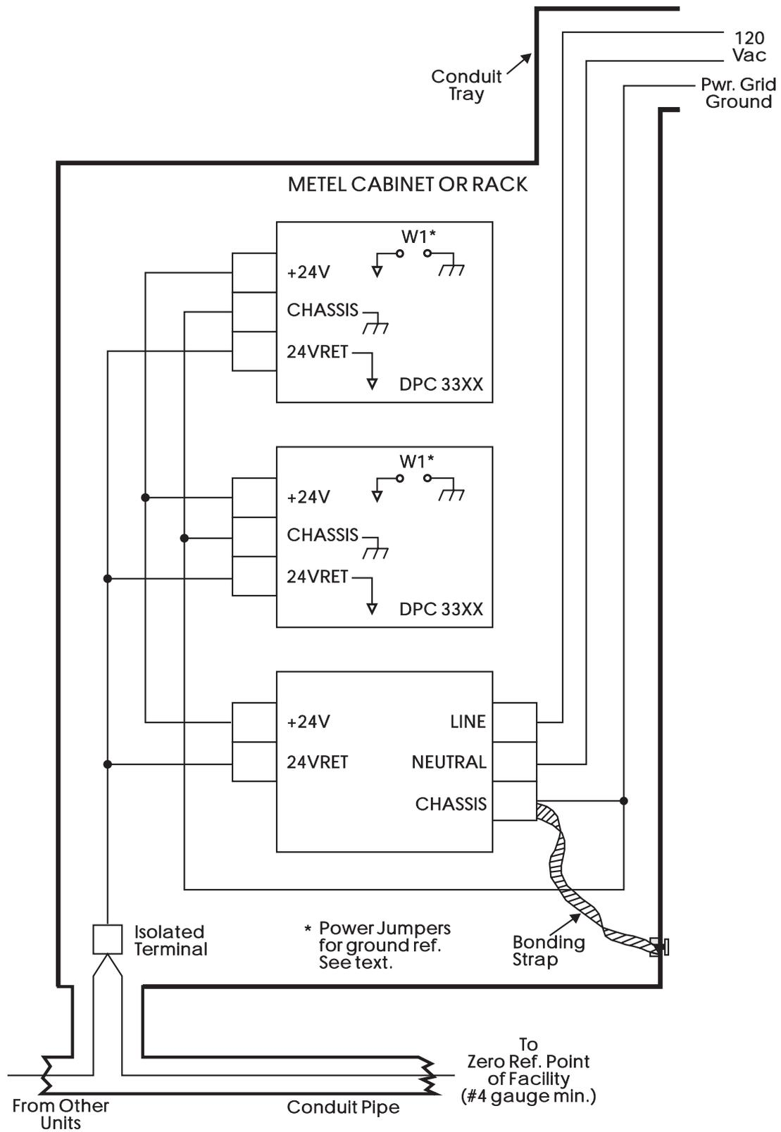
**Figure 8 Grounding for DPCs and Power Supplies in Single Metal Cabinet**
