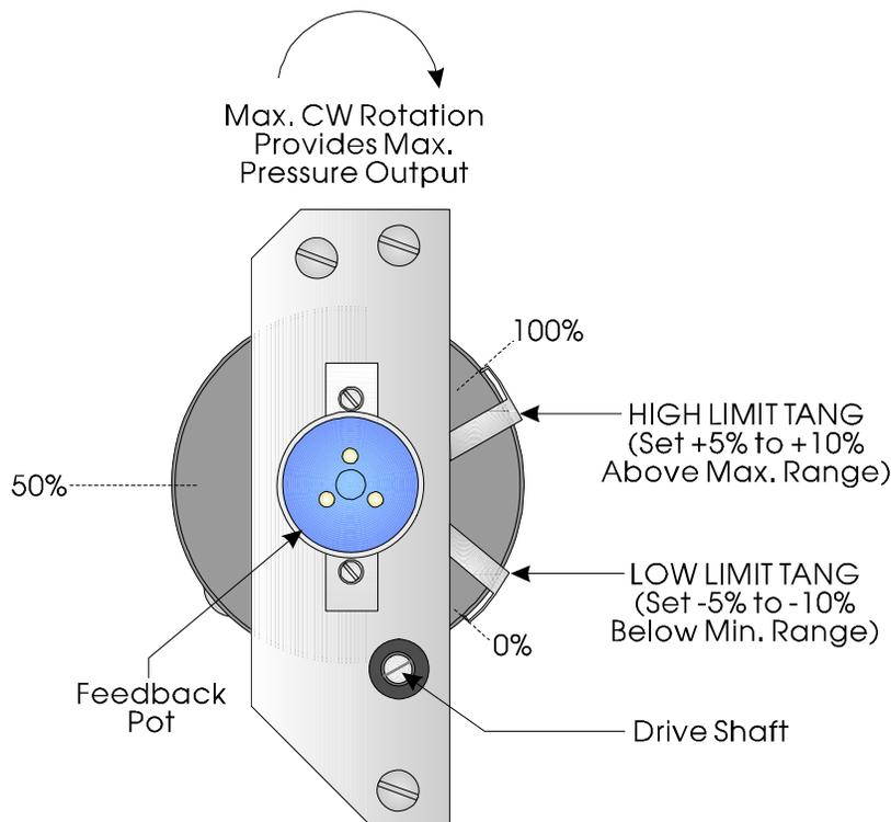
**Figure 5-1 - Rear View of Gear Drive Assembly**
