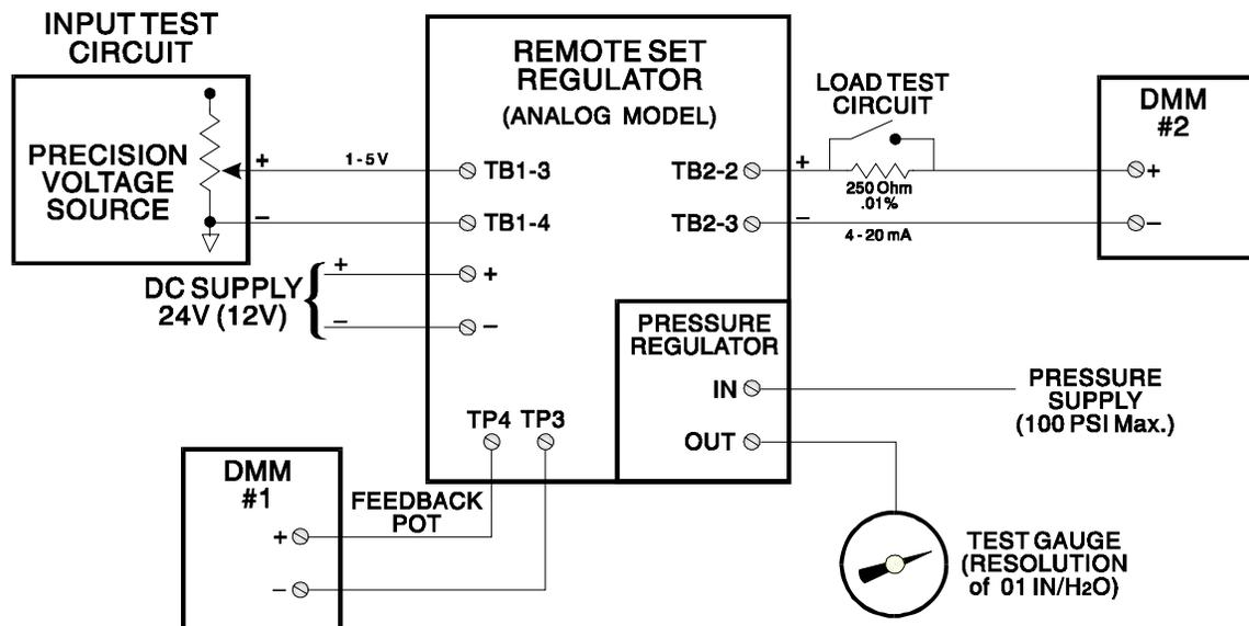
Figure 5-2 - Analog Test Setup
