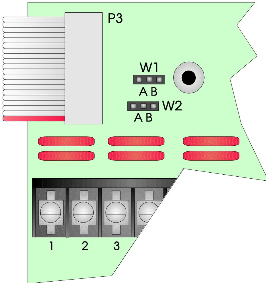
**Figure 3-2 - Jumper Location on Analog Termination Board**
