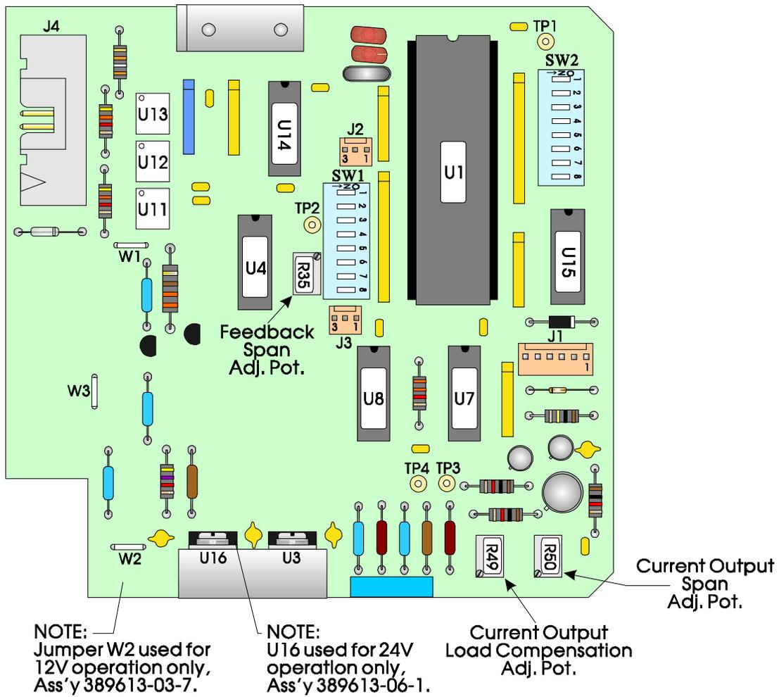
Figure 5-6 - Assembly, Raise/Lower Type CPU Board with Current Output
