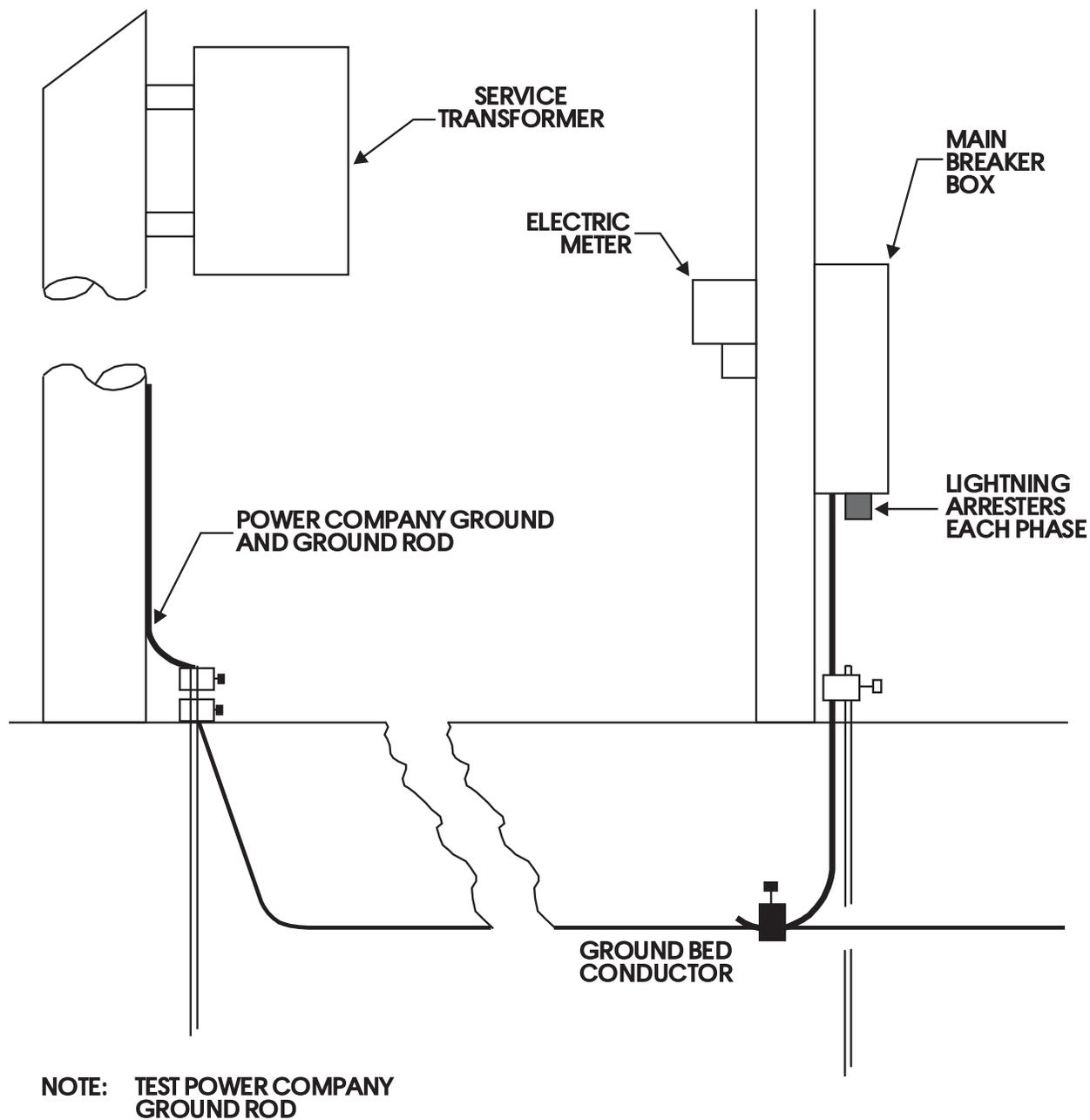
Figure 7 AC Power Grounding System
