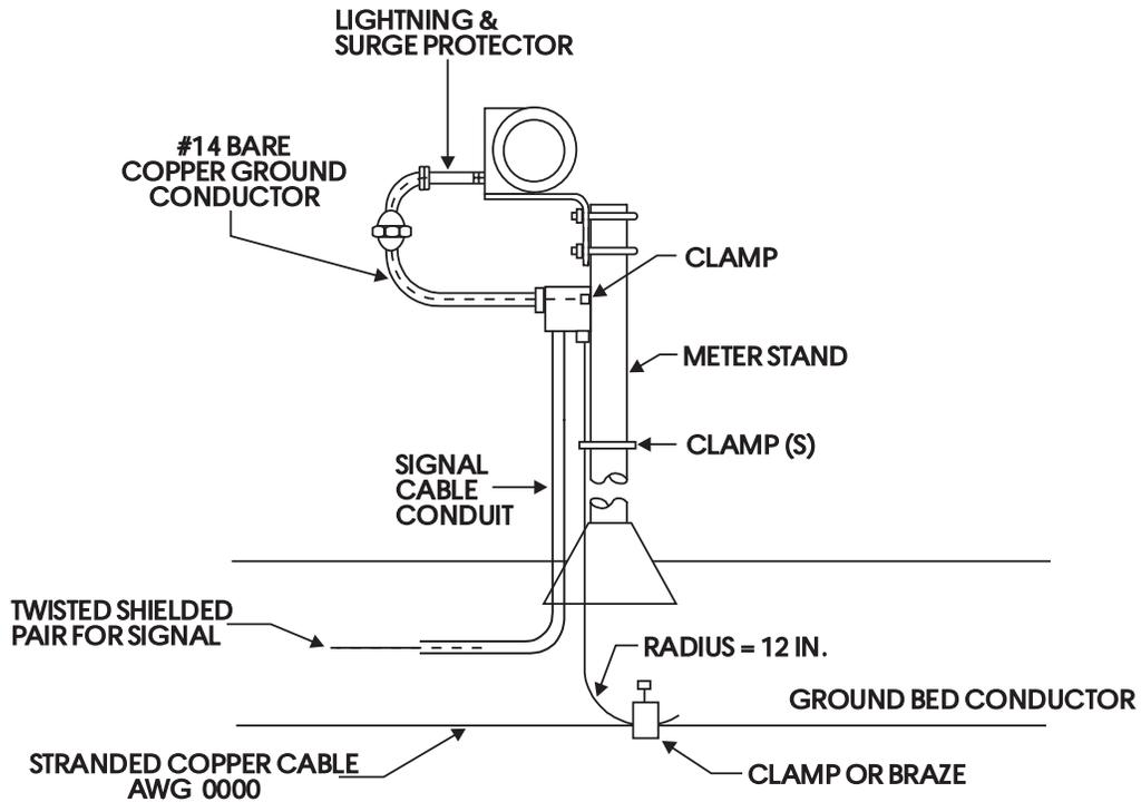
Figure 5 Grounding of Transmitter
