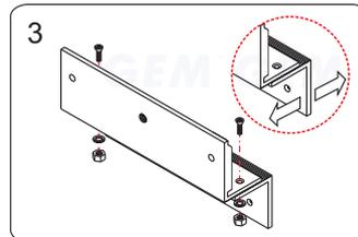
3 Assemble the Z bracket, and make sure that the Z bracket is adjustable.
