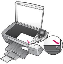
**c** Place the photo (face down) on the right front corner of the glass. Make sure the long edge of the photo is along the front of the glass. Close the lid.
