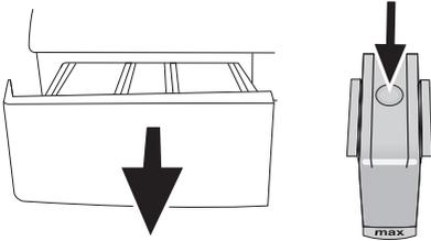
1. If more than a normal amount of water and softener mixture starts to gather in the softener compartment, the siphon must be cleaned.
