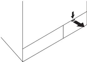
the tab on the filter cap downwards and pull the piece out towards yourself. If it is composed of one piece, hold it from both sides and open it by pulling out.
