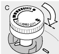
5. Turn the steam regulator ④ clockwise to the end of the red marking (B) and then 6. keep turning it to the double-arrow marking ⇄. The steam regulator will lift (C).
