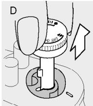
7. Pull out the steam regulator together with the valve vertically (D). Do not touch the lower end of the anti-calc. valve with your fingers, to avoid a possible greasy film.
