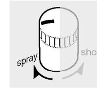
**Spray** (coming from the nozzle ③): The spray function can be used at any temperature, to dampen laundry. To do so, press the button ⑥ (water spray = blue).
