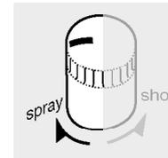
**Spray / shot of steam 2-function button:** The functions «water spray» and «shot of steam» can be activated with a 2-function button. The desired function can be selected by turning the button ⑥ as far as it will go. The marking (blue = water spray or red = shot of steam) must point to the respective function (e). Turn the button from blue (spray) to red (shot of steam) anti-clockwise and from red to blue clockwise (e).
