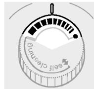
**Steam regulator ④:** Select the quantity of steam required (c) for each garment with the steam regulator ④. You can increase the quantity by turning the steam regulator clockwise (wide markings) to the end of the red marking.
