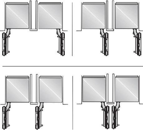
If there is a partition with a thickness **from  $\frac{5}{8}$ " (16 mm) to  $6 \frac{5}{16}$ " (160 mm)** between the adjacent appliances, then each appliance should be individually installed within its own niche using the mounting accessories included.
