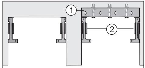
If the installation niche is deeper than the appliance, a solid wooden beam ① can be placed behind the anti-tip brackets ② so the appliance can be securely attached to the base or wall.
