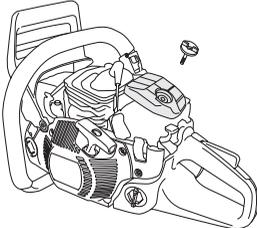
The filter can be cleaned more thoroughly by washing it in water and detergent.
