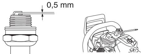
**Note!** Always use the recommended spark plug type! Use of the wrong spark plug can damage the piston/cylinder. Check that the spark plug is fitted with a suppressor.
