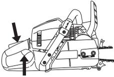
**CAUTION!** Do not pull the starter cord all the way out and do not let go of the starter handle when the cord is fully extended. This can damage the machine.
