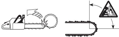
Cutting with the bottom edge of the bar, i.e. from the top of the object downwards, is known as cutting with a pulling chain. In this case the chain saw pulls itself towards the tree and the front edge of the chain saw body rests naturally on the trunk when cutting. Cutting with a pulling chain gives the operator better control over the chain saw and the position of the kickback zone.
