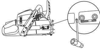
The chain is correctly tensioned when it does not sag from the underside of the bar, but can still be turned easily by hand. Hold up the bar tip and tighten the bar nuts with the combination spanner.
