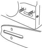
Tension the chain by turning the chain tensioning screw clockwise using the combination spanner.
