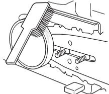
Regularly check that the brake band is at least 0.024 inch (0.6 mm) thick at its thinnest point.
