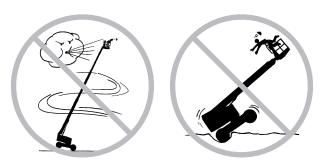
Use extreme care and slow speeds while driving the machine in stowed position across uneven terrain, debris, unstable or slippery surfaces and near holes and drop-offs. Do not drive the machine on or near uneven terrain, unstable surfaces or other hazardous conditions with the boom raised or extended.
