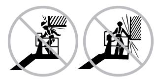
Be aware of crushing hazard when grasping the platform guard rail.
