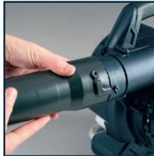
5. Push the assembled blower tube over the discharge port and rotate until locks in place and the screw hole can be seen.
