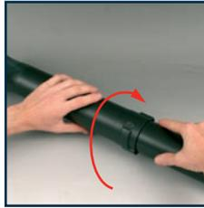
3. Rotate the nozzle tube clockwise locking it into place.
