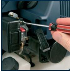
**IMPORTANT.** Blower tubes and intake cover must be installed while adjusting engine idle speed. Engine idle speed will also be affected if either the intake cover or blower tubes are blocked, damaged or incorrectly installed.
