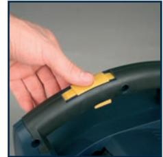
Move the sliding throttle lock to central position.
