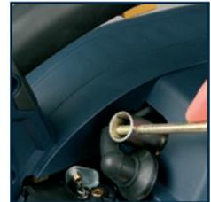
3. Clean and adjust the spark plug gap to 0.6 - 0.7mm. Replace any damaged or visibly worn plug with a CHAMPION CJ8, NGK BM6A or equivalent spark plug.
