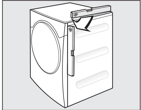
The dryer must be perfectly level to ensure safe and proper operation.
