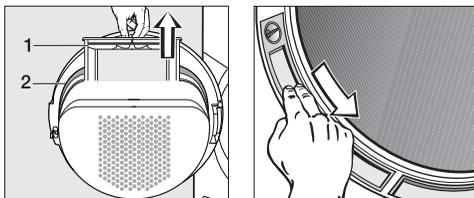
The fluff filters located in the door and the door opening collect fluff from items being dried.
