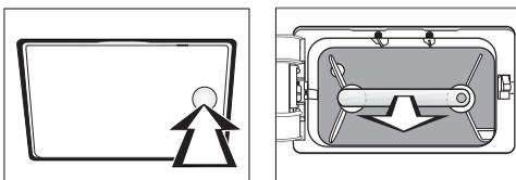
The fine filter is behind the service panel on the bottom left. It collects finer fluff, hair and detergent residues which have got through the surfaces of the fluff filters in the door and the door opening.
