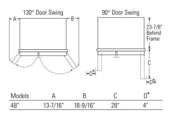
\* Four inch (4") minimum clearance is required when door swing is adjusted to 90°. If the 90° door stop position is used, drawer access is maintained, but drawer removal is restricted.
