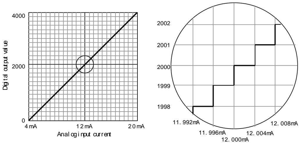
Figure 1.6 A/D conversion characteristic ( 4 ~ 20mA )
