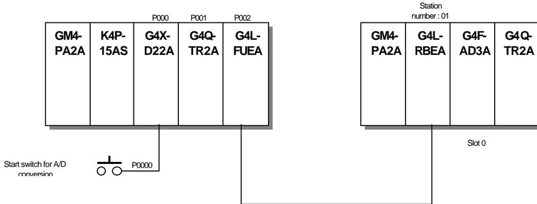
Fnet communication module on self-station : slot 2
