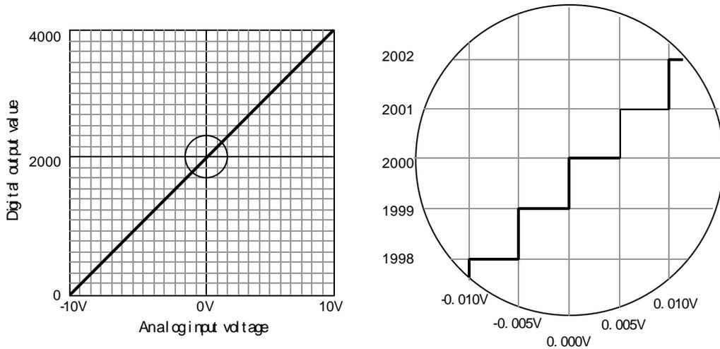
Figure 1.5 A/D conversion characteristic (-10 ~ 10VDC)
