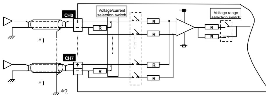
\*1: Use a two-core twisted pair shielded cable
