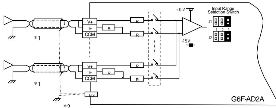
\*1: Use a two-core twisted pair shielded cable
