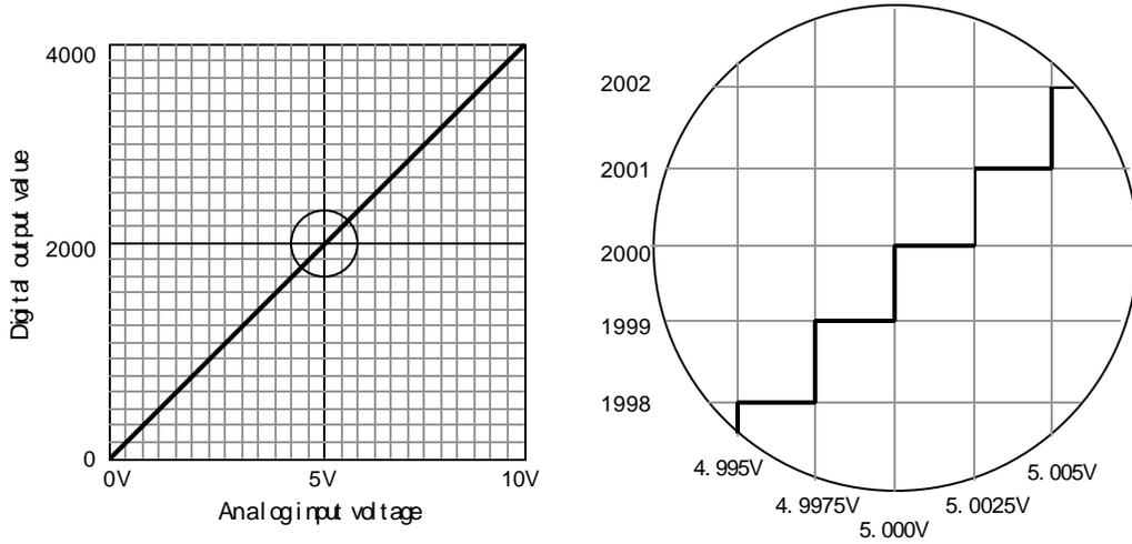
Figure 1.4 A/D conversion characteristic (0 ~ 10VDC)
