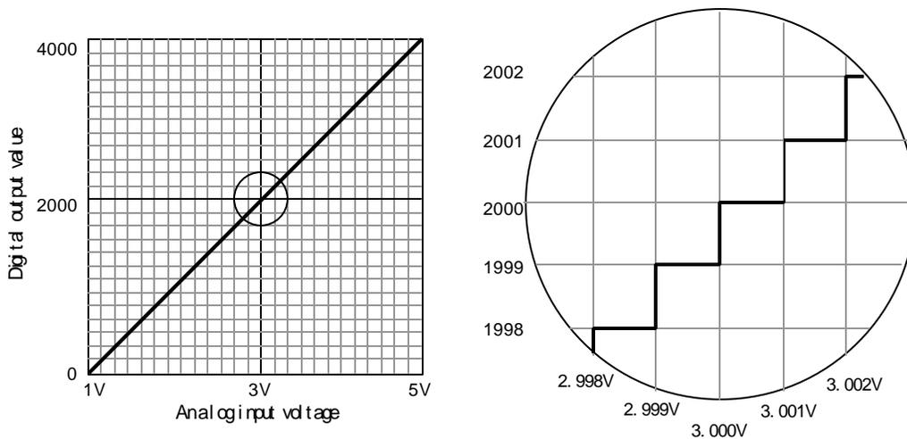
**Figure 1.3 A/D conversion characteristics ( 1 ~ 5VDC )**
