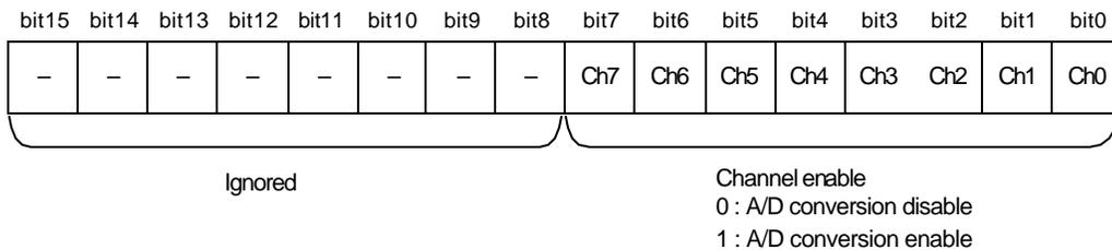
Example) To enable channel 1, 2, and 3 for G4F-AD3A :
