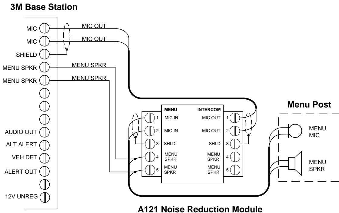
**Figure 1. Wiring for 3M C760/960/1060 Base Station**
