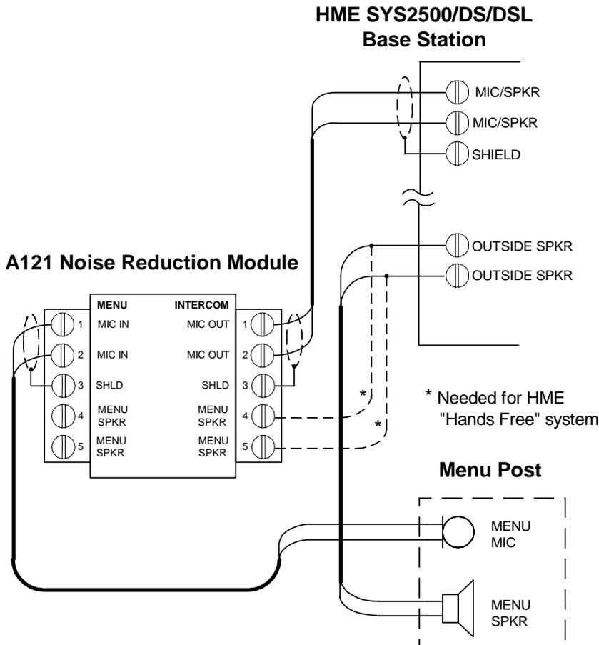
**Figure 7. Wiring for HME SYS2500/DS/DSL Base Station**
