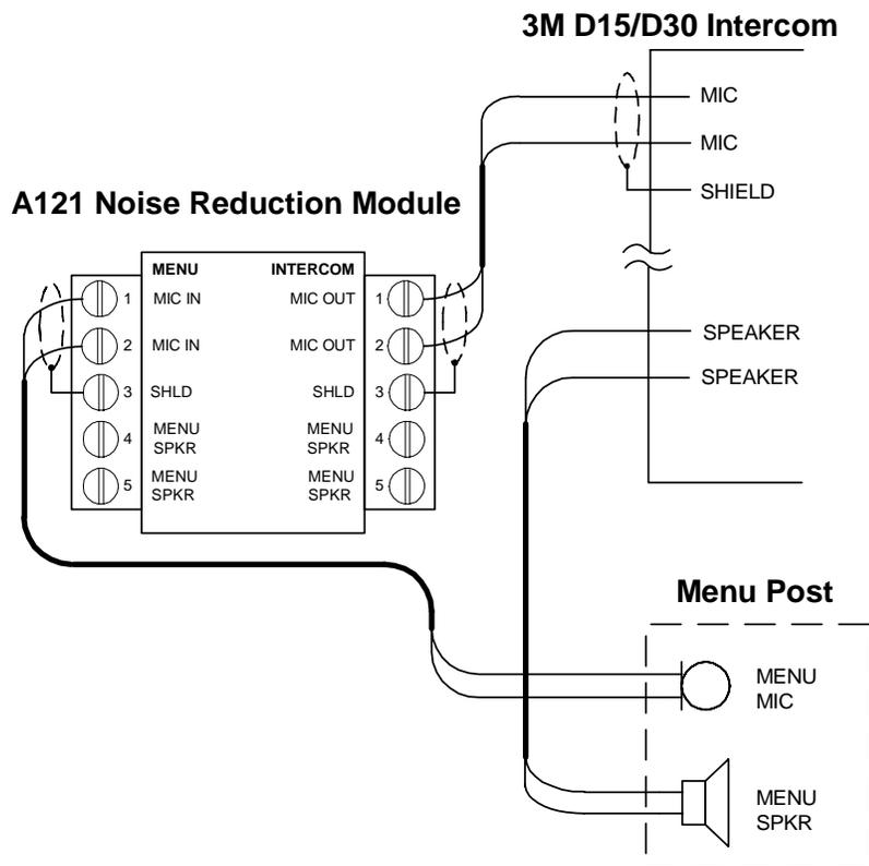
Figure 4. Wiring for 3M D15/D30 Intercom
