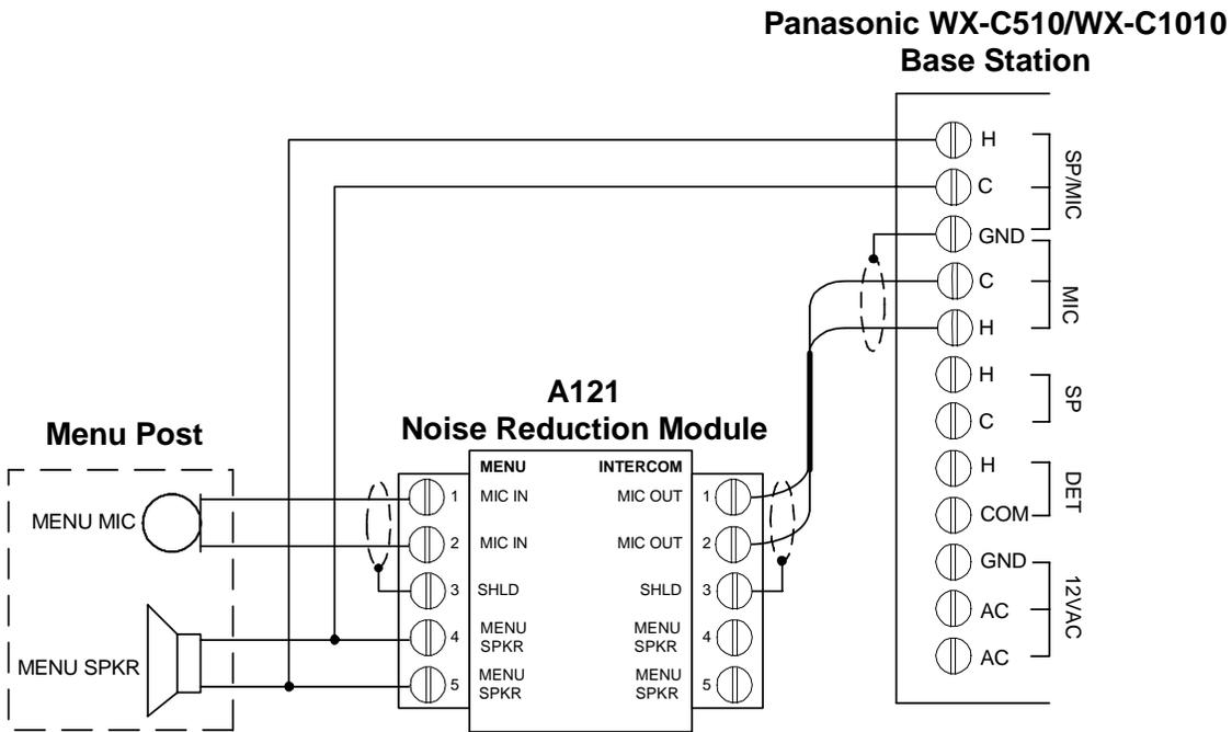
**Figure 6. Wiring for Panasonic WX-C510/WX-C1010 Base Station**
