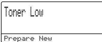
The machine is supplied with the Standard TN-110 toner cartridge that must be replaced after approximately 2,500 pages (Black) and 1,500 pages each (Cyan, Magenta and Yellow). When a toner cartridge is running low, the LCD shows `Toner Low`. (For details about the specific order number for each toner cartridge color by page yield, see *Ordering accessories and supplies* on page iii.)
