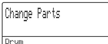
The machine uses a drum unit to create print images on paper. If the LCD shows `Change Parts Drum`, the drum unit is near the end of its life and it is time to buy a new one.
