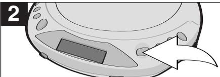
While the unit is off, press the PLAY/PAUSE (▶||)/POWER ON button to start playback. To **pause PLAYBACK**, press the PLAY/PAUSE (▶||)/POWER ON button again, the display will blink. Press once again to resume playback.
