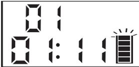
If no more vibration occurs, the music signals are once again stored into the memory and the indicator returns to full. When the memory is full, the top bar will blink and the disc rotation speed will drop to save power consumption.
