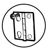
Loosen top screw from each hinge on the dryer face half way. With one hand holding the top of the door and the other hand holding the bottom, remove the door from the dryer by lifting it **UP** and **OUT**.
