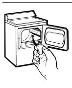
Before replacing the light bulb, be sure to unplug the dryer power cord or disconnect the dryer at the household distribution panel by removing the fuse or switching off the circuit breaker. Reach above dryer opening from inside the drum. Remove the bulb and replace with the same size bulb.
