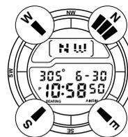
4. Next, you can adjust the rotary direction bezel so that the "N" or "N" mark is aligned with the magnetic north indicator. This correctly aligns all of the markings on the bezel.
