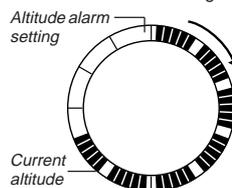
The graphic display would appear as illustrated here when your current altitude is 700 meters, after you set the altitude alarm for 1,000 meters and the initial measurement was 0 meters. Note that seven segments of the graph are darkened because you are 7/10 of the way to the value set for the altitude alarm.
