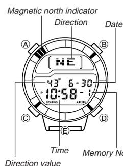
While in the Digital Compass Mode, use (D) to scroll through the data in the following sequence.
