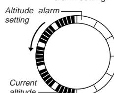
The graphic display would appear as illustrated here when your current altitude is 1,500 meters, after you set the altitude alarm for 1,000 meters and the initial measurement was 2,000 meters. Note that five segments of the graph are darkened because you are 5/10 of the way to the value set for the altitude alarm.
