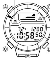
1. In the Altimeter Mode, hold down (D) until the watch emits a short beep, indicating the start of the measurement.
