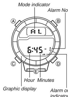
Five independent daily alarms can be set. Each alarm lets you set the hour and minutes. When the Daily Alarm is on, the alarm sounds for 20 seconds at the preset time each day. Press any button to stop the alarm after it starts to sound. When the Hourly Time Signal is on, the watch beeps every hour on the hour.
