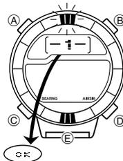
1. While in the Digital Compass Mode (Normal screen), hold down (A) until the upper display changes to show "-1-".
