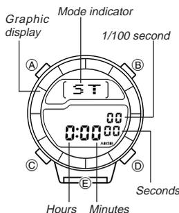
The Stopwatch Functions let you measure elapsed time, split times, and two finishes. The range of the stopwatch is 23 hours, 59 minutes, 59.99 seconds.
