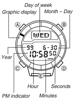
You can set the time and date in the Timekeeping Mode, which you can enter using (C). In the Timekeeping Mode, the graphic display shows counting of the seconds.
