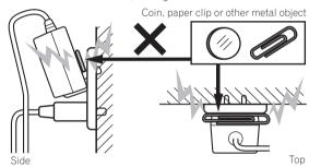
The power plug could come detached from the AC adapter and remain in the power outlet if someone trips on the AC adapter's power cord or if something hits the AC adapter. If this happens, remove the power plug remaining in the outlet with dry hands, holding it as shown on the diagram below and without touching metal parts. Do not use any tools to remove it.
