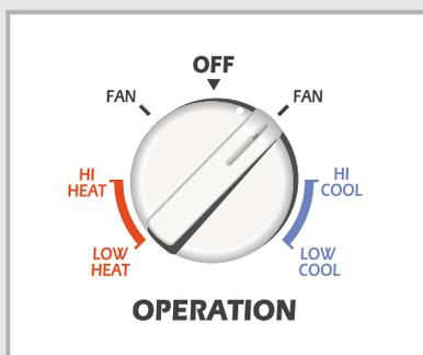
*If the atmosphere in your room is stale, you can air it using the Fan feature and if necessary, evacuate the stale air outside.*
