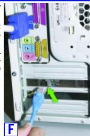
The Adapter's installation is complete. Next, you must install the Adapter's device drivers. Refer to Step 2 to use the Setup Utility CD or the section for your Operating System on the back of this Quick Installation.
