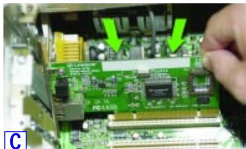
**Important:** When installing the Adapter, be sure to press it solidly into the PCI slot. The Adapter is built to resist the pressure necessary to insert it correctly in the PCI slot. Avoid a call to technical support by making sure that the Adapter is inserted all the way into your PC's PCI slot. You will know this has occurred when the Adapter's faceplate is flush with your computer's slot.
