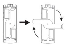
1. Before using the tuner, rotate the support bar clockwise. Make certain the unit is stable before extending and rotating the antenna rods.
