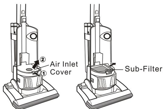
**Caution:** Do not wash the sub-filter in a washing machine, and do not use any other equipment such as a hair dryer to dry it. Always allow 24 hours for drying. Do not operate the vacuum without the sub-filter. Be sure the sub-filter is dry and properly installed. Failure to do so could result in electrical shock, personal injury, or motor failure.
