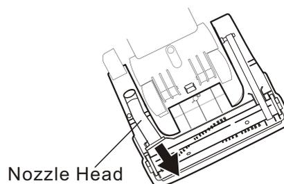
**Caution:** When the suction hose A, B or Nozzle head is blocked, the bypass valve will be opened automatically to protect the motor, resulting in the suction force being reduced. The bypass valve will be at its original position automatically after the blockage is removed.
