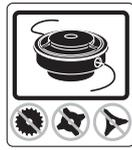
Only use non-metallic, flexible cutting elements, that is trimmer head with trimmer cord.
