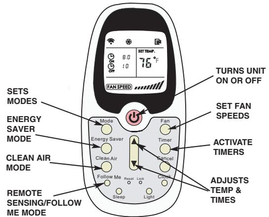
Fig. "B" REMOTE CONTROL w/DISPLAY & REMOTE SENSING/FOLLOW ME BUTTON
