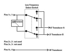
**Three way Mode:** The internal -6dB per octave network in **NOT** applied to either LF transducer. Shading is accomplished with signal processing. The switch handle points to the side of the non-shaded (full range) low-frequency transducer ONLY IF the full range signal is applied to pins 1+ and 1- and the shaded signal to pins 2+ and 2-. Default position for three way mode is position A; if put in position B, connections to LF transducers A and B are interchanged.
