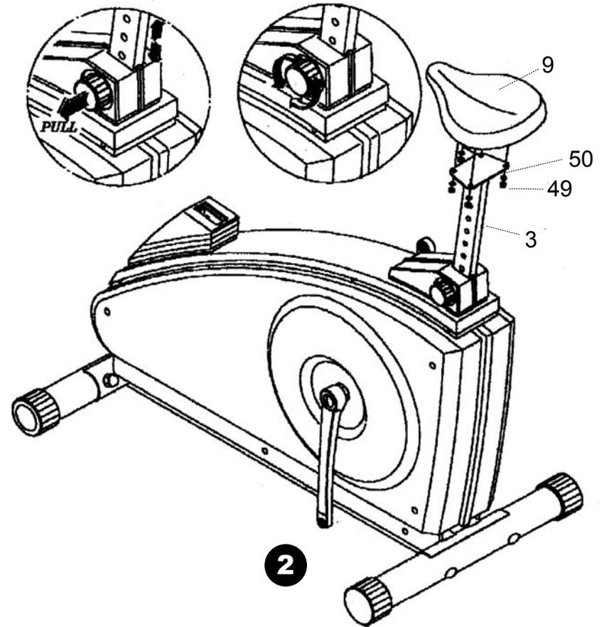
2. Attach the seat (9) to the seat post (3) with the locknuts (49) and flat washers (50) already provided on the underside seat bolts.
