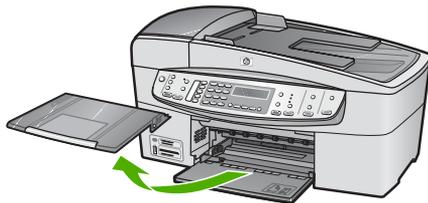
2. Slide the paper-width guide to its outermost position.
