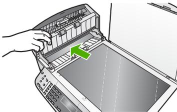
5. Lower the automatic document feeder mechanism, and then close the cover of the automatic document feeder.
