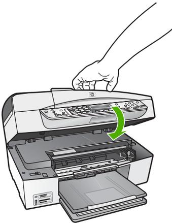
9. If you installed a new print cartridge, the print cartridge alignment process begins.
