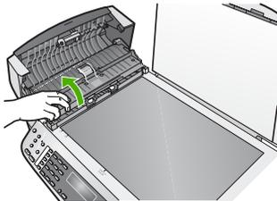
4. Check for any paper jammed in the automatic document feeder mechanism.
