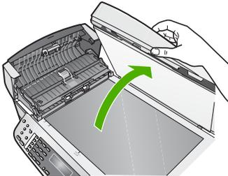
4. Lift the automatic document feeder mechanism.
