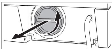
Clean the filter under a tap, to remove any traces of fluff.
