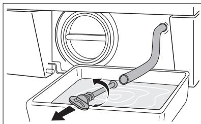
7. When no more water comes out, unscrew the pump cover by turning it anti-clockwise and remove the filter. Use pliers, if necessary. Always keep a rag nearby to dry up any water spillages when removing the cover.
