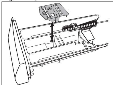
5. Clean all parts of the washing machine, especially the nozzles in the top of the washing-in chamber, with a brush.
