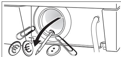
9. Check carefully whether the pump impeller rotates (it rotates jerkily). If it doesn't rotate, please contact your Service Centre.
