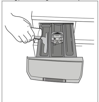
2. If required, pour fabric softener into the compartment marked
