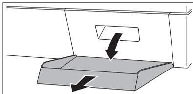
6. Pull out the emergency emptying hose, place it in the container and remove its cap.
