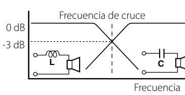
$$L = \frac{159 \times R}{f_c} \text{ (mH)} \quad C = \frac{159000}{f_c \times R} \text{ (μF)}$$
