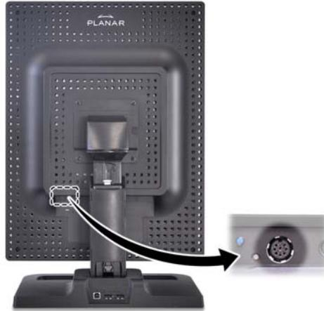
*Input power port on connector plate*
