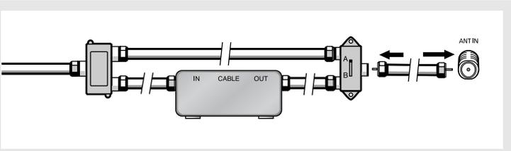
After you've made this connection, set the A/B switch to the “A” position for normal viewing. Set the A/B switch to the “B” position to view scrambled channels. (When you set the A/B switch to “B,” you will need to tune your TV to the cable box's output channel, which is usually channel 3 or 4.)
