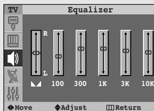
◀ "Equalizer" is not available when the "BBE" function is activated ("On").
