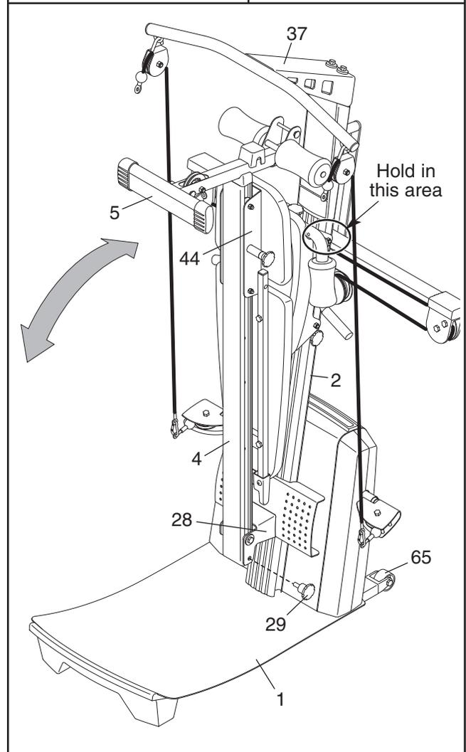
**⚠ WARNING:** Make sure that Storage Knob (29) is in place and fully tightened each time the resistance system is used.
