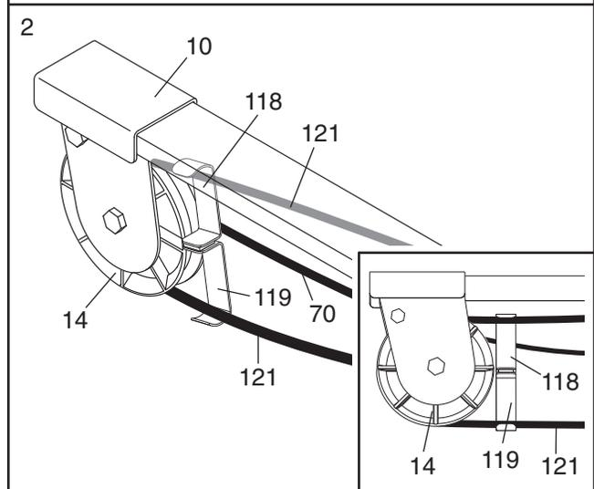
Slide the Tension Gauges (118, 119) next to the Large Pulley (14) as shown in the inset drawing.
