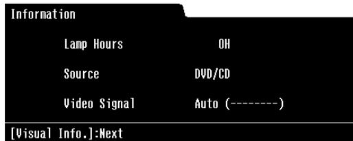
**Note:** If the lamp has been used less than 11 hours, 0H is displayed.
