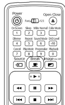
**Note:** After 5 minutes in break mode, the lamp turns off and the screen darkens. After 30 minutes, the power shuts off, and you need to press the
