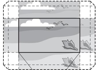
2. Rotate the zoom ring to reduce or enlarge the picture.
