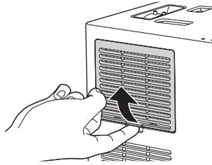
4. Remove the old filter and install the new filter.
