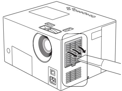
3. If you need to replace the filter, press up on the tab and lift off the cover.
