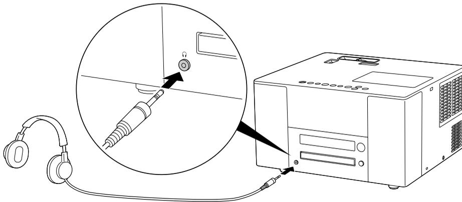
After you connect headphones, you no longer hear any sound from the built-in speakers or the optional subwoofer. However, you can still adjust the volume to the headphones using MovieMate's volume controls on the control panel or remote control.
